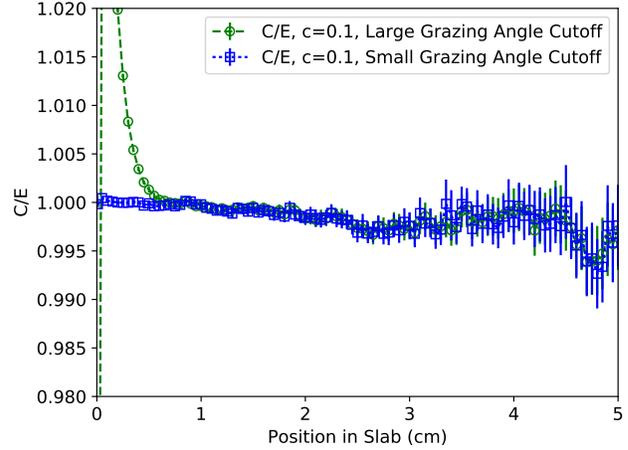
Fig. 2. Comparison of analytic results for Benchmark 3.1.2 with MCNP6 results for two grazing angle cutoffs.
