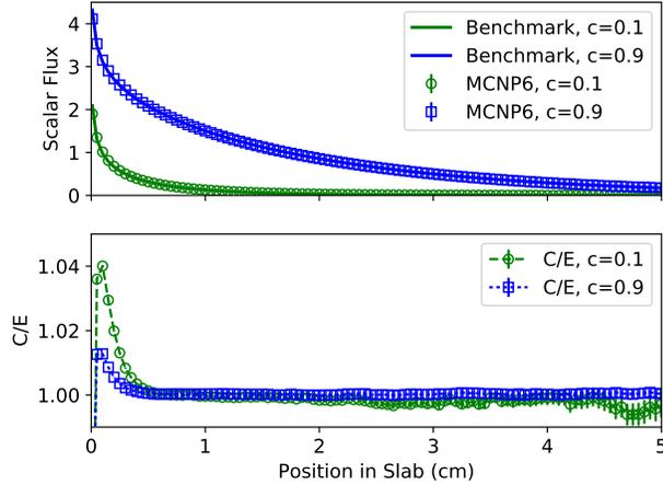
Fig. 1. Comparison of analytic results for Benchmark 3.1.2 with MCNP6 results for an isotropic source.
