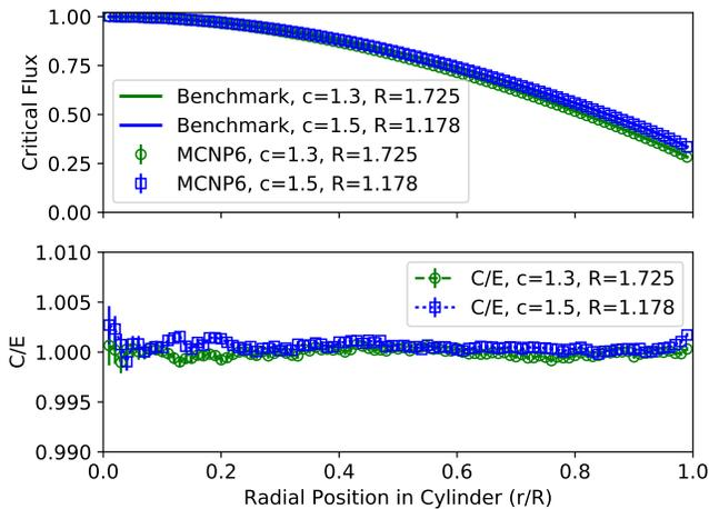
Fig. 3. MCNP6 values divided by the analytic solution for Benchmark 3.4.2 with a volume source for two values of  $c$  and radii.
