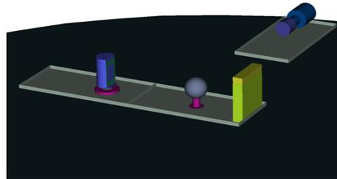
Fig. 1. Modeled BeRP Ball Experimental Measurement Configuration
