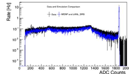
Fig. 4. Comparison of  $^{137}\text{Cs}$  spectra measured with an HPGe detector and calculated with MCNP using ENDF version 7 data
