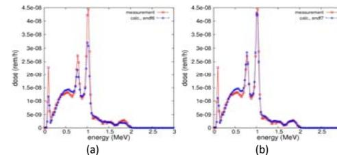
Fig. 3. Comparison of measured doses with calculated doses from a DU sphere using (a) ENDF version 6 and (b) ENDF version 7
