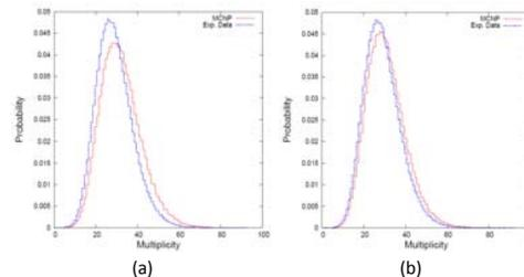
Fig. 2. Comparison of multiplication curves obtained using (a) ENDF data and (b) modifications to the ENDF data within uncertainties that improve agreement to benchmark measurements
