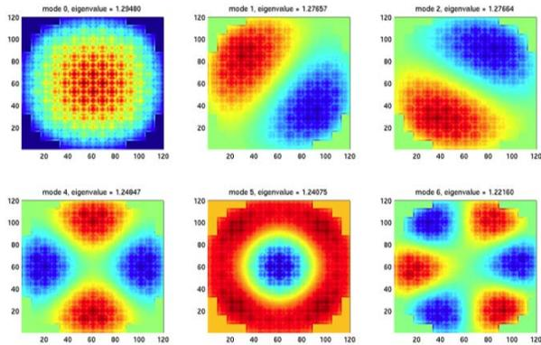
Fig. 1. Some eigenmodes for a 2-D PWR.
