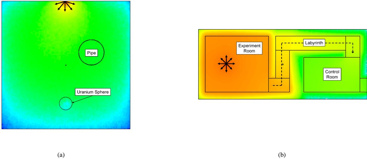
Fig. 3. (a) Photon flux distribution of the neutron on ground problem. (b) Neutron flux distribution of a criticality accident.
