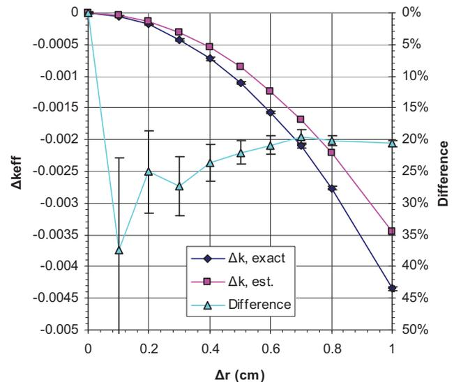
Fig. 2. The change in  $k_{eff}$  as a function of the translation of the  $^{235}\text{U}$  sphere.  $1\sigma$  error bars are shown in all figures.
