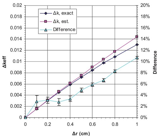
Fig. 3. The change in  $k_{eff}$  as a function of the “bulging” displacement of the right side of the  $^{235}\text{U}$  sphere.
