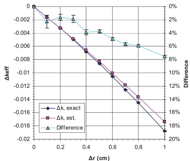
Fig. 4. The change in  $k_{eff}$  as a function of the “collapsing” displacement of the left side of the  $^{235}\text{U}$  sphere.
