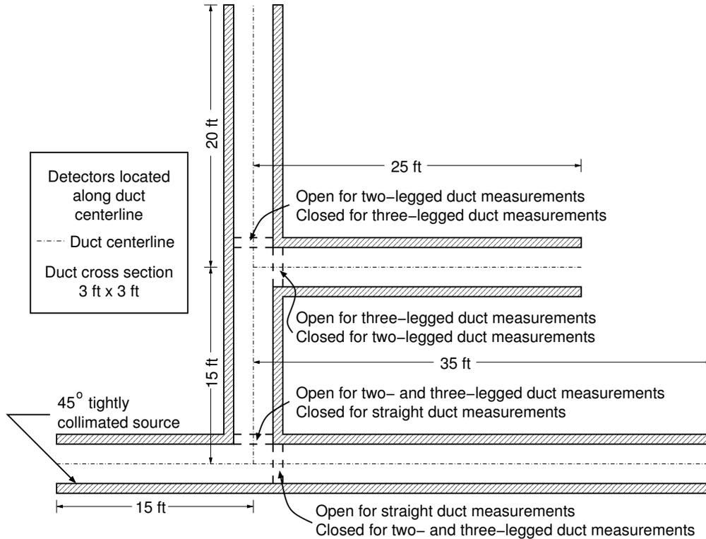
Fig. 1. Three duct problem geometry—specific paths are closed off to create the desired duct shape (adapted from [2])
