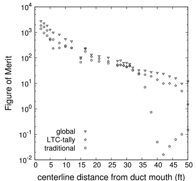
Fig. 3. Tally figure-of-merit comparisons for the three-legged duct
