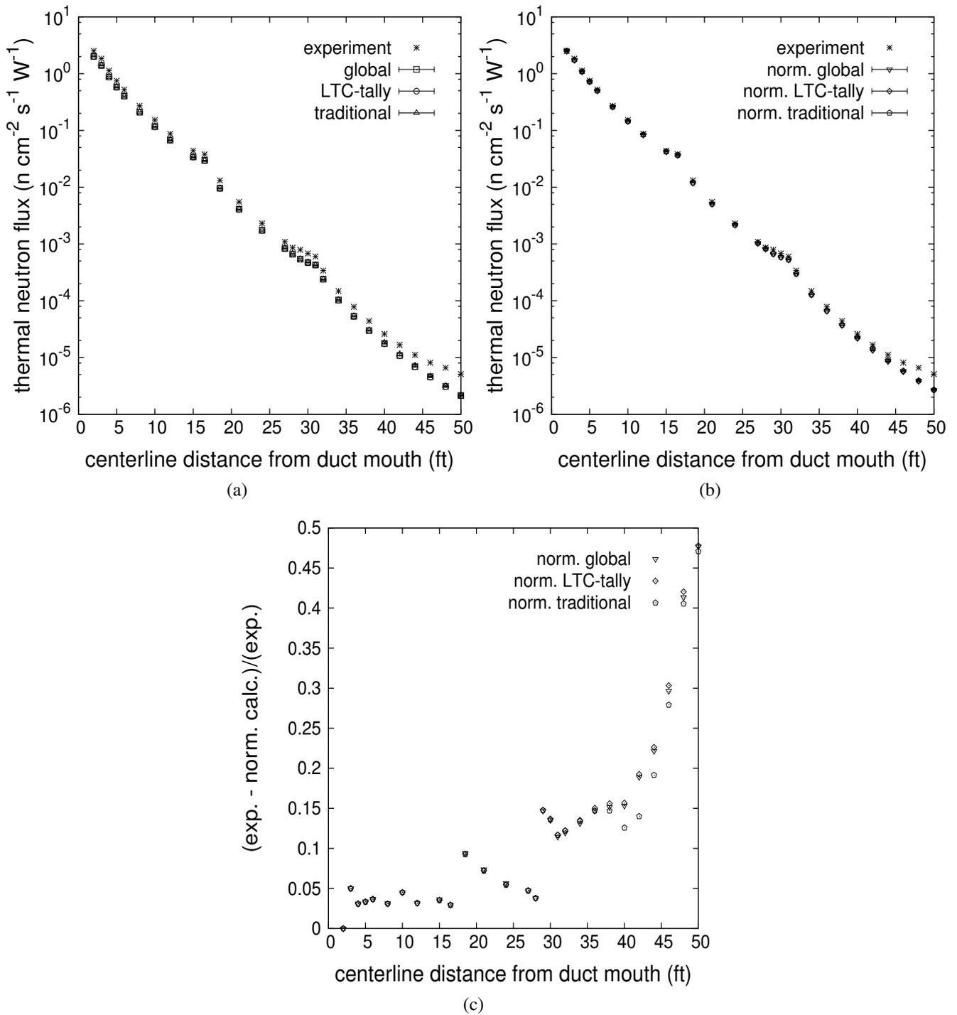
Fig. 2. (a) Comparison of three-legged duct computed results to experimental results, (b) comparison of three-legged duct normalized results to experimental, and (c) relative error in normalized computed results
