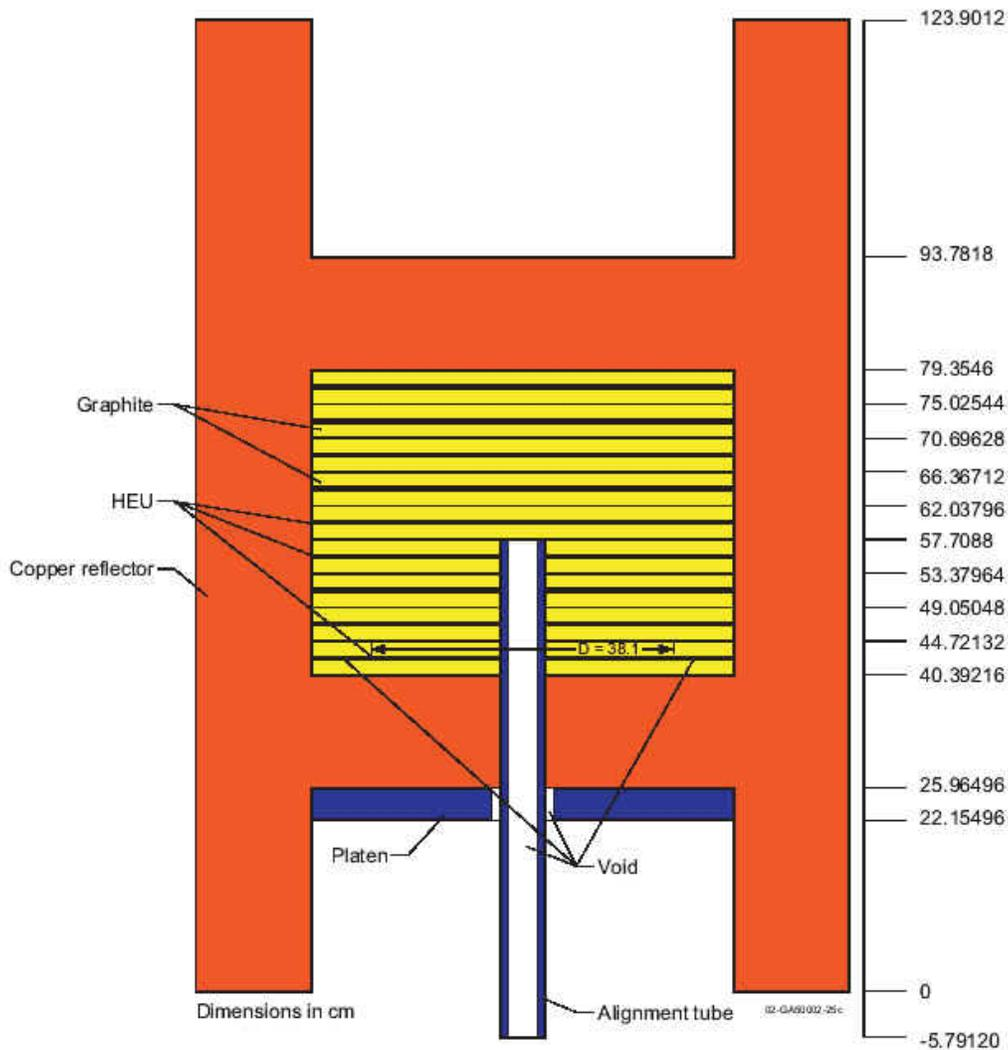
**Figure 4. Vertical slice through the benchmark model of the third Zeus assembly**
