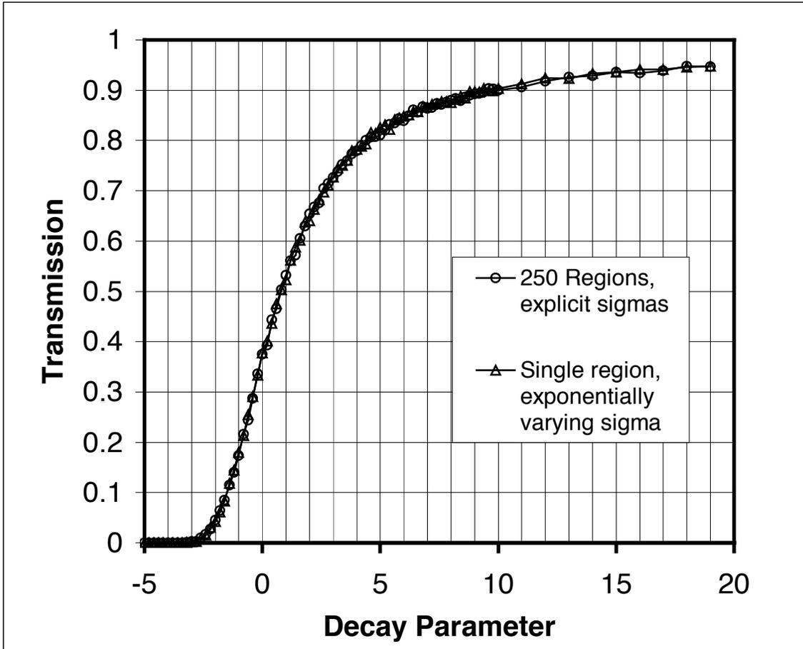
Figure 1. Transmission through a 1 mfp thick infinite slab as a function of cross-section decay parameter. Direct sampling from continuously varying cross-section compared with 250 regionwise cross-sections.
