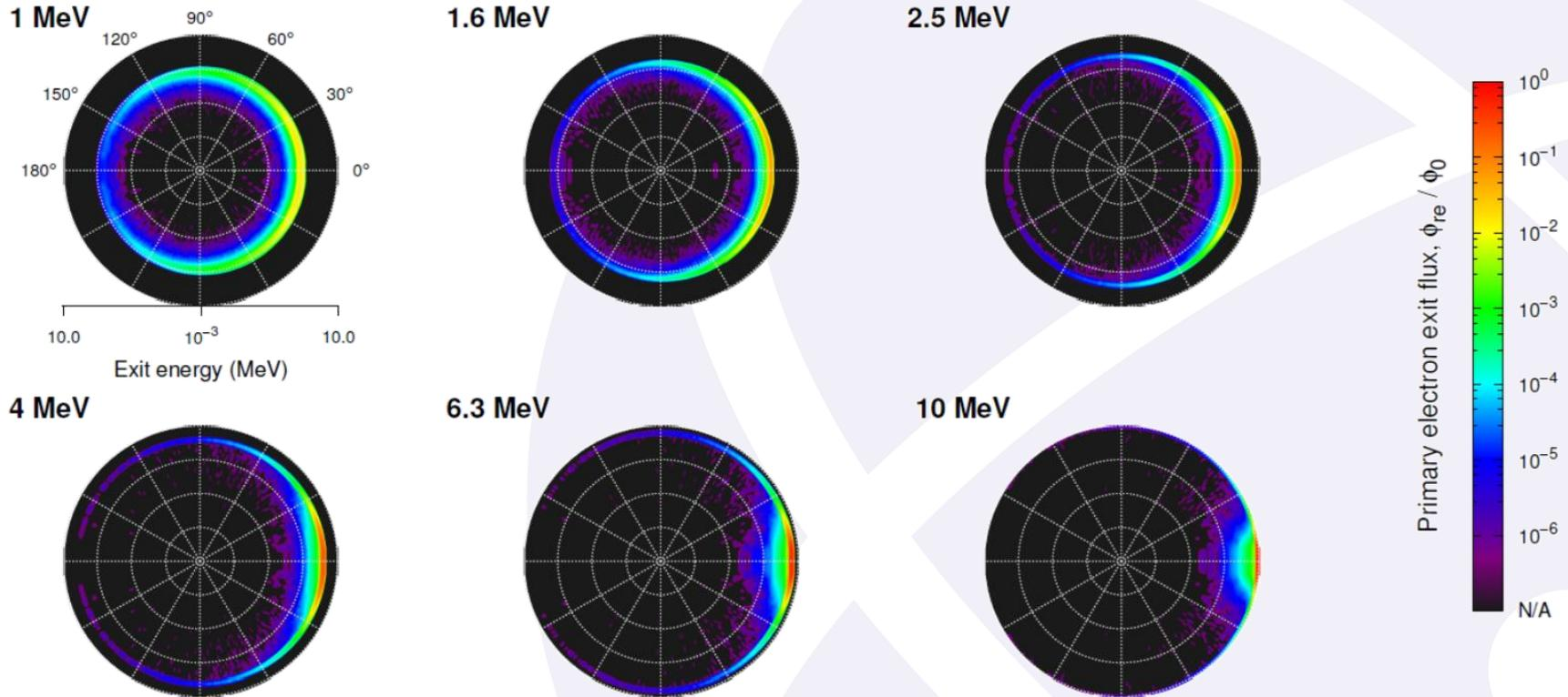
*Energy and angle-resolved exit fluxes of primary/incident runaway electrons colliding with a Ne pellet fragment with indicated initial energy.*
