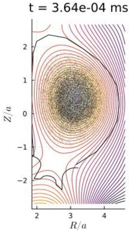
Runaway wall impact during a vertical displacement event (VDE).
