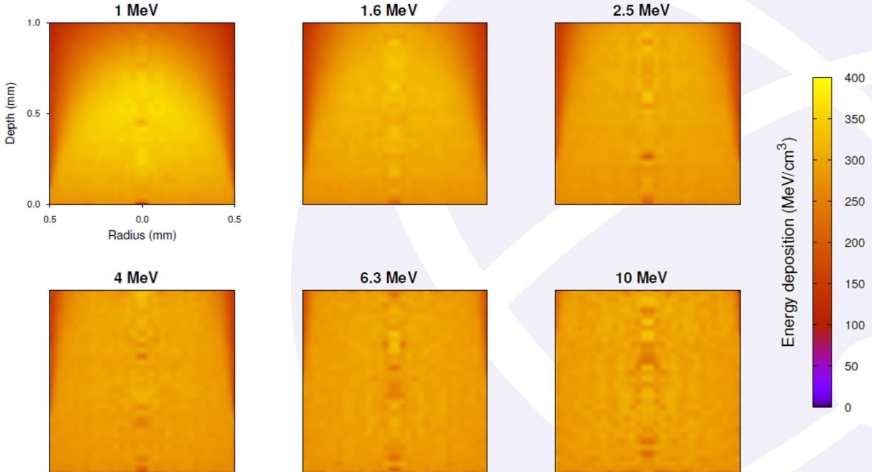
*Volumetric energy deposition distributions from incident runaway electrons into Ne pellet fragments with indicated initial energy.*
