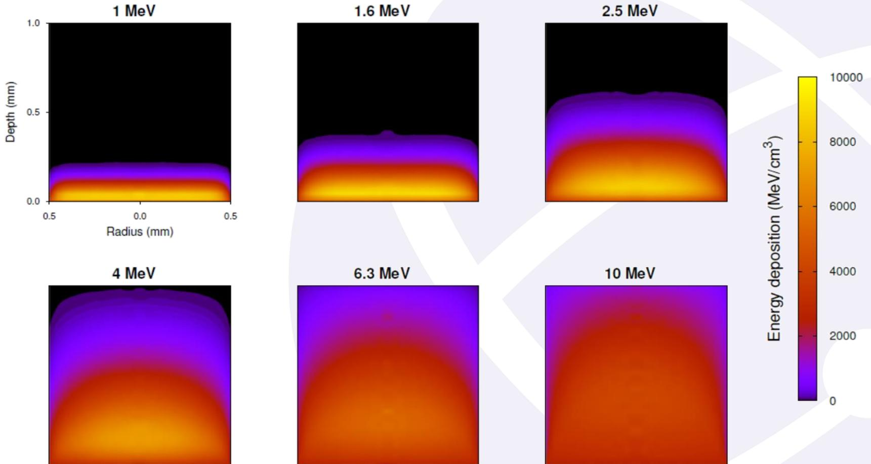
*Volumetric energy deposition distributions from incident runaway electrons into W particulates with indicated initial energy.*
