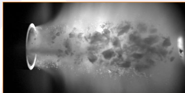
Cryogenic D-Ne shattered pellet exiting an injection system at 250 m/s (ORNL, 2021).
