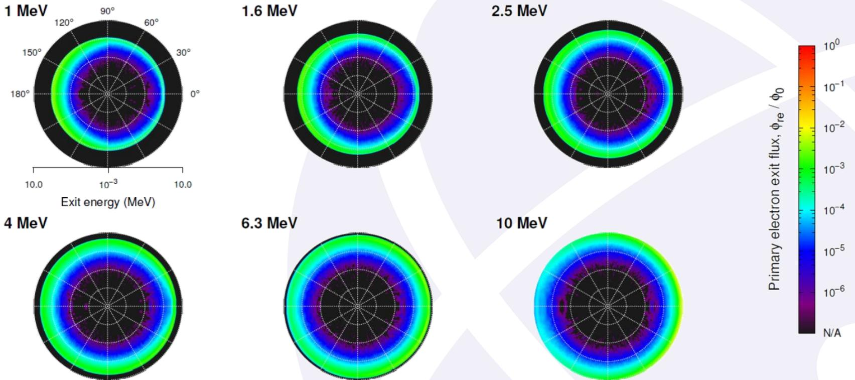
*Energy and angle-resolved exit fluxes of primary/incident runaway electrons colliding with a W particulate with indicated initial energy.*
