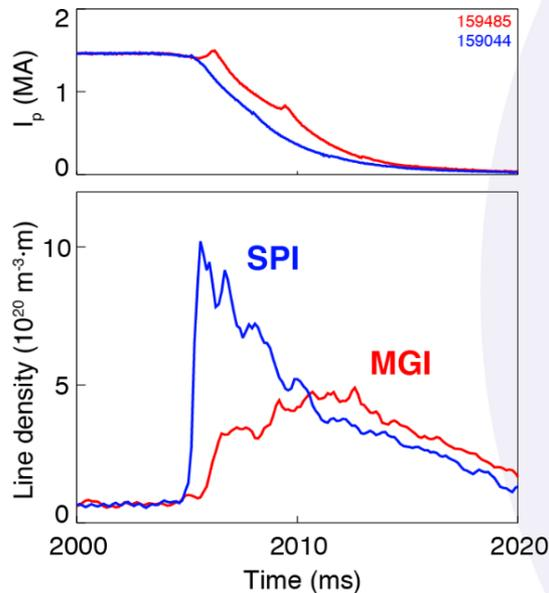
FIG. 1. Comparison of line integrated densities during the CQ for equivalent neon SPI and MGI injections.
