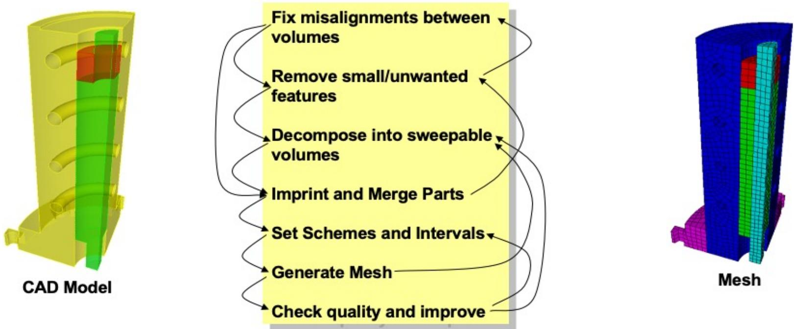
The CAD to mesh process can be a complex series of iterative steps requiring in-depth understanding of the model and its flaws, expertise in using the software, and creativity to infer and apply solutions.
