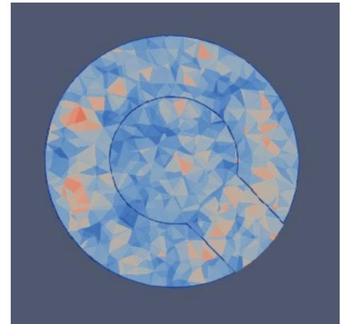
UM models with linear tet, hex, and/or mixed hex/pent elements are typically used in MCNP UM calculations.
