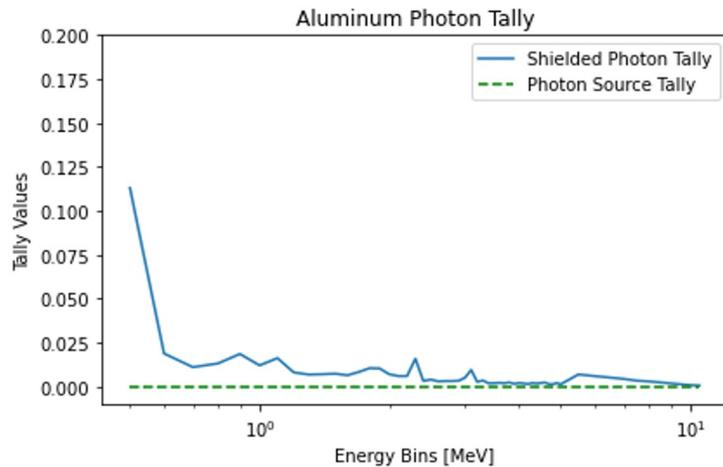
F1 photon tally results. Photons generated from neutron inelastic scattering.
