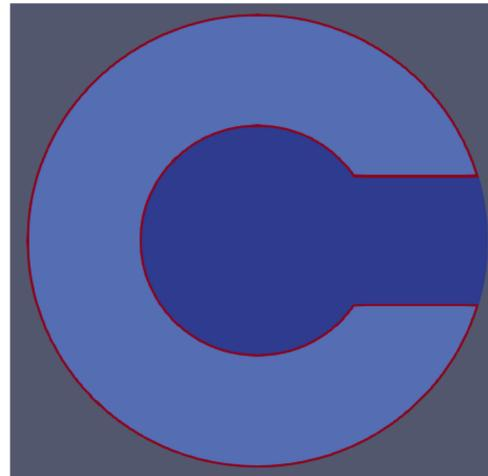
Oktavian geometry cross section, red borders are steel, interior dark blue is air and light blue ring composed of aluminum powder
