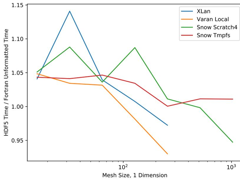
Figure 1: HDF5 vs. Unformatted IO Performance
