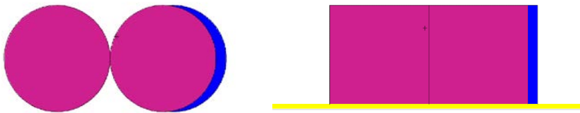
Figure 8. MCNP6.2 top and side view illustrations, respectively, of model geometry. Pu metal-water mixture is shown in magenta; water in blue and steel in yellow.
