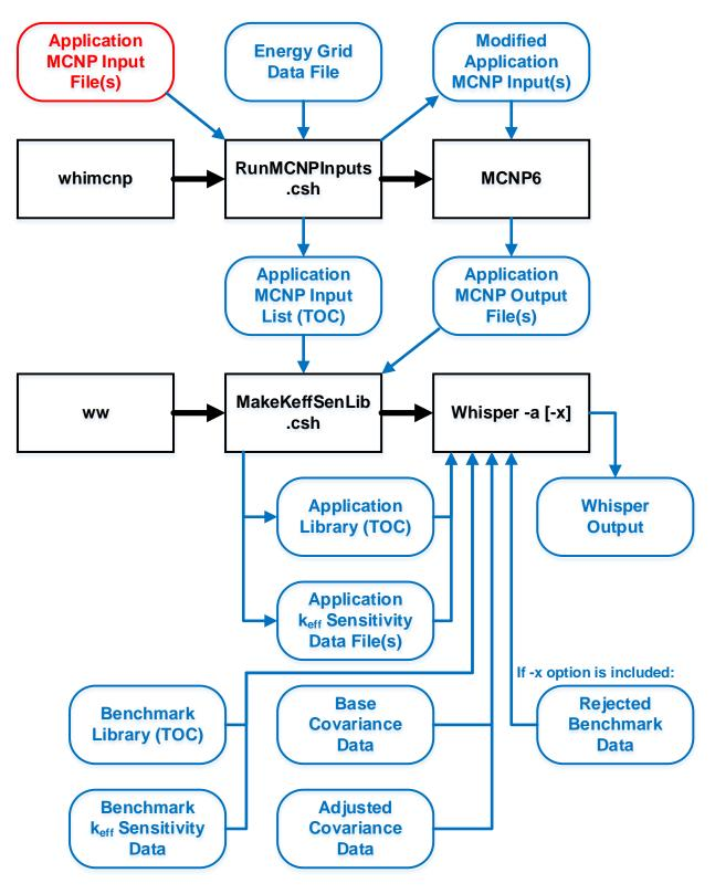
Figure 1 Application Model Evaluation Flowchart
