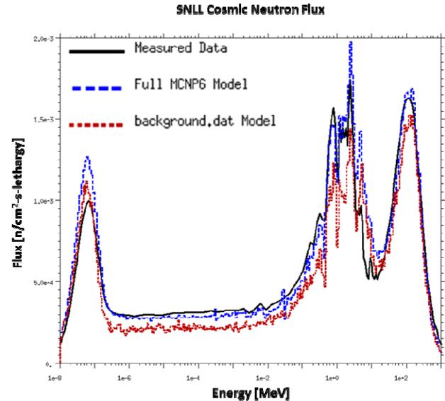
**Fig. 2.** Measured (black) neutron flux spectra for Nov. 6, 2006 at SNLL (37.7°N, 122.7°W), Livermore, CA. Simulations used 38°N, 120°W with elevation and date adjusted on the SDEF card. The full MCNP6 model (blue) incorporated all building and structural materials, while the background.dat simulation (red) included only soil and concrete on the ground.
