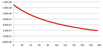
Figure 3. First 192 eigenvalues for 2D PWR problem, using a 120x120 spatial mesh for fission matrix tallies.
