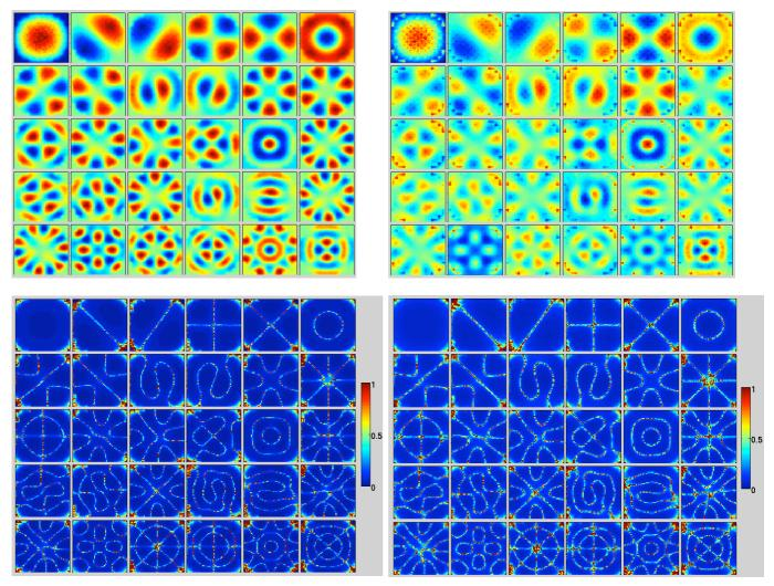
Figure 5. First 30 forward flux modes (top) of 2D PWR and relative uncertainties (bottom), Group 1 (0.625 eV – 20 MeV).
