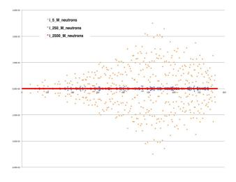
Figure 8. Detail for imaginary parts of 2D PWR eigenvalues, after 5M, 250M, and 2500M neutrons. (vertical scale: -6x10<sup>-3</sup> to +6x10<sup>-3</sup>)
