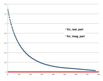
Figure 7. Real and Imaginary parts of the 772 eigenvalues for the 2D PWR problem, using a 30x30 spatial mesh for fission matrix tallies.
