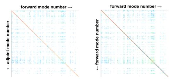
Figure 10. Biorthogonality of forward and adjoint fission source modes (left), and orthogonality of forward modes (right). Plotted points are inner products of modes. (scales: red - near 1.0, blue ≤ 0.1)
