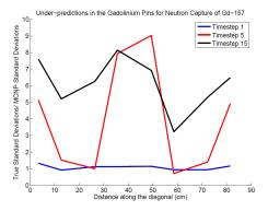
Fig. 3. Uncertainty under-prediction for <sup>157</sup>Gd capture as a function of space at various time steps.
