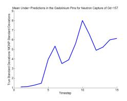
Fig. 4. Uncertainty under-prediction for <sup>157</sup>Gd capture as a function of time averaged over all space.
