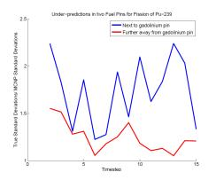
Fig. 5. Uncertainty under-prediction for <sup>239</sup>Pu fission as a function of time with different proximity to burnable poison (gadolinium) pin.
