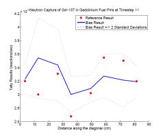
Fig. 2. Comparison of reference and biased results for <sup>157</sup>Gd capture.
