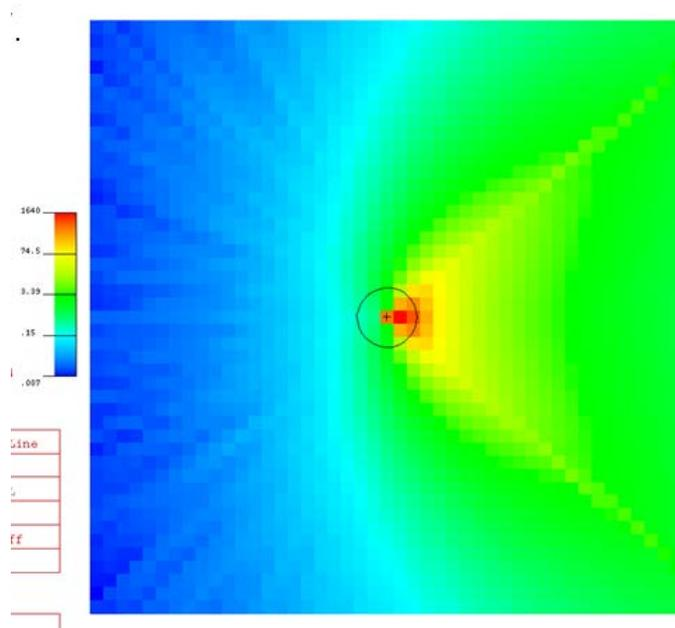
Figure 2. Mesh tally plot of low-energy photons with Cerenkov cone.
