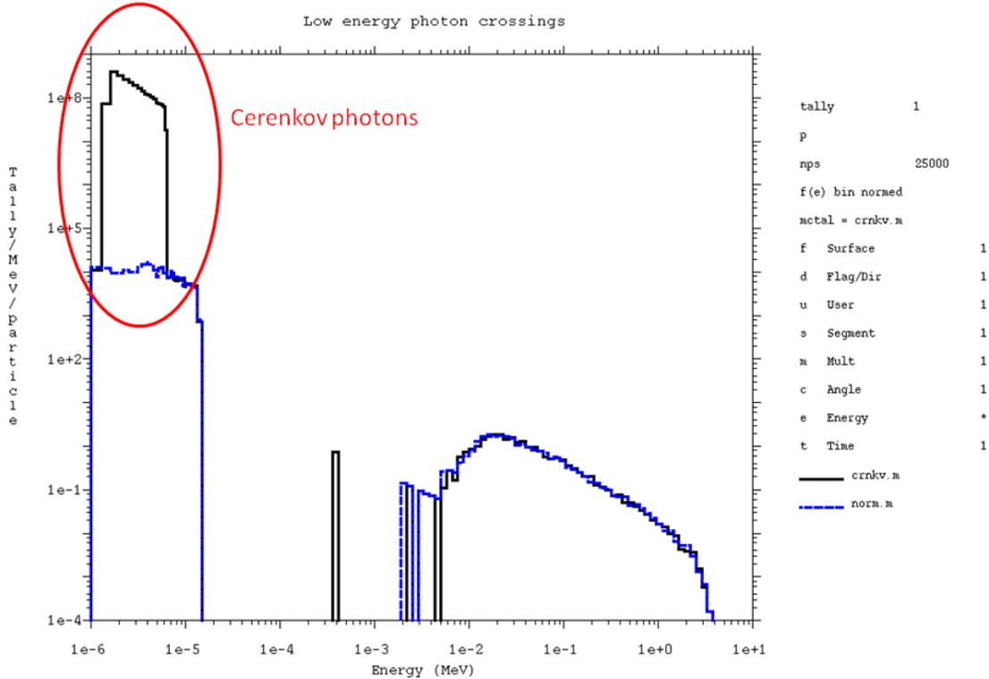
Figure 1. Plot of low-energy photons showing Cerenkov photon production.
