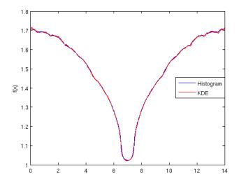
Fig. 4. Comparison of flux profiles obtained from histogram and KDE collision tallies for the continuous-energy problem.
