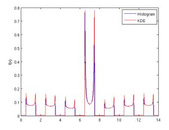
Fig. 6. Comparison of absorption reaction rate profiles obtained from histogram and KDE collision tallies for the continuous-energy problem.
