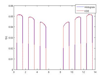
Fig. 2. Comparison of fission reaction rate profiles obtained from histogram and KDE collision tallies for the one-group problem.
