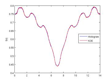
Fig. 1. Comparison of flux profiles obtained from histogram and KDE collision tallies for the one-group problem.
