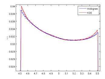
Fig. 7. Comparison of fission reaction rate in one slab of fissionable material for the continuous-energy problem.
