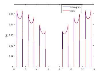
Fig. 5. Comparison of fission reaction rate profiles obtained from histogram and KDE collision tallies for the continuous-energy problem.
