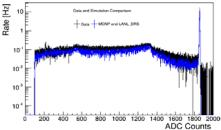
Fig. 4. Comparison of <sup>137</sup>Cs spectra measured with an HPGe detector and calculated with MCNP using ENDF version 7 data
