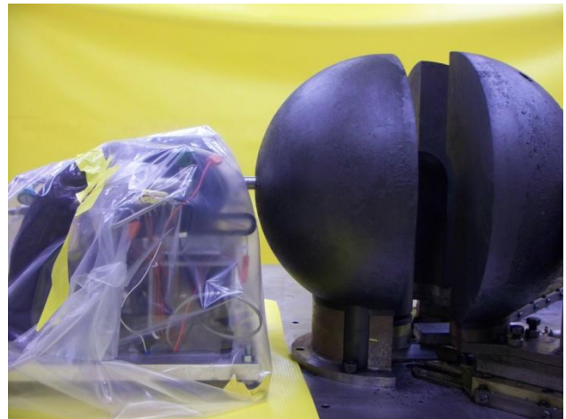
Figure 1. Side view of the Flat-Top assembly with the heat pipe. The assembly is shown in the SCRAM position.
