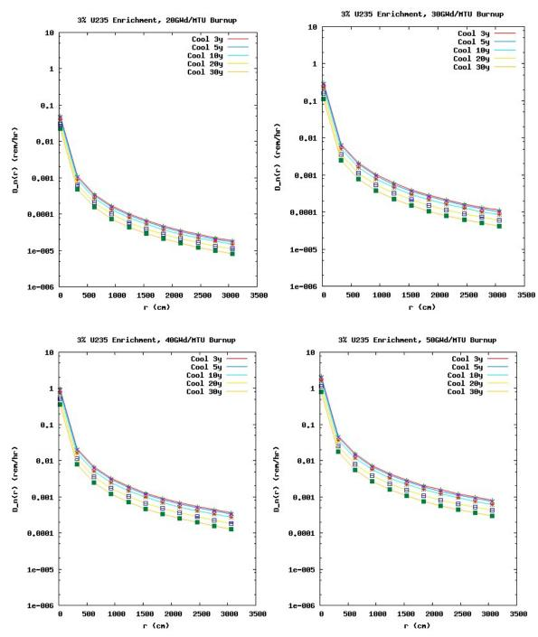
Figure 8. Neutron dose rate as a function of distance for 3% <sup>235</sup>U enrichment; 20, 30, 40, and 50 GWd/MTU burnup; and 3, 5, 10, 20, and 30 year cooling following irradiation.
