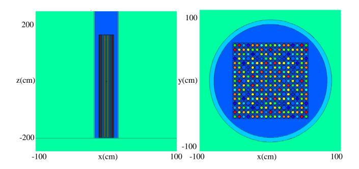
Figure 7. MCNP6 geometry plots of the 0.32-m-diameter chemical processing model showing fuel assembly, nitric acid (blue), and air (green).
