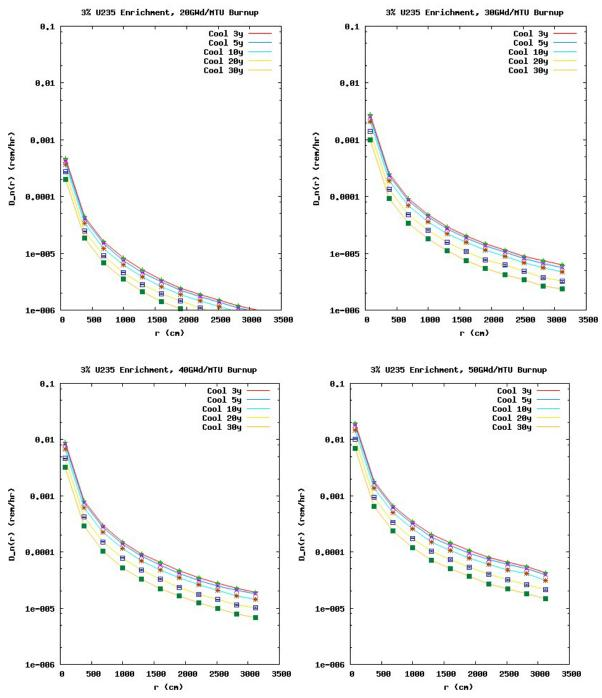
Figure 3. Neutron dose rate as a function of distance for 3% <sup>235</sup>U enrichment; 20, 30, 40, and 50 GWd/MTU burnup; and 3, 5, 10, 20, and 30 year cooling following irradiation.
