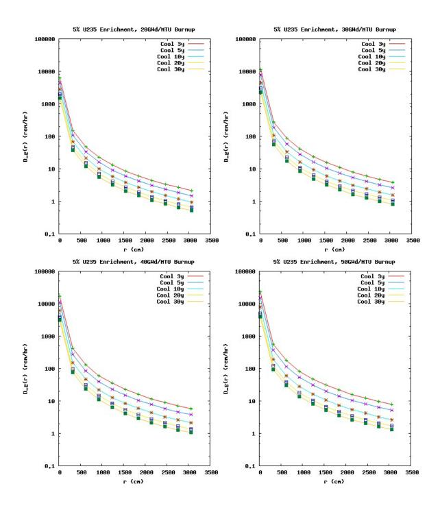
Figure 11. Photon dose rate as a function of distance for 5% <sup>235</sup>U enrichment; 20, 30, 40, and 50 GWd/MTU burnup; and 3, 5, 10, 20, and 30 year cooling following irradiation.
