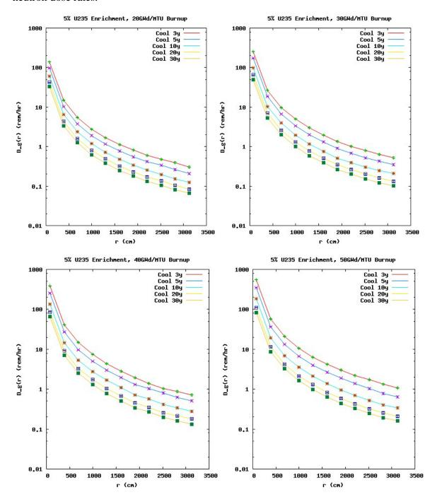
Figure 6. Photon dose rate as a function of distance for 5% <sup>235</sup>U enrichment; 20, 30, 40, and 50 GWd/MTU burnup; and 3, 5, 10, 20, and 30 year cooling following irradiation.
