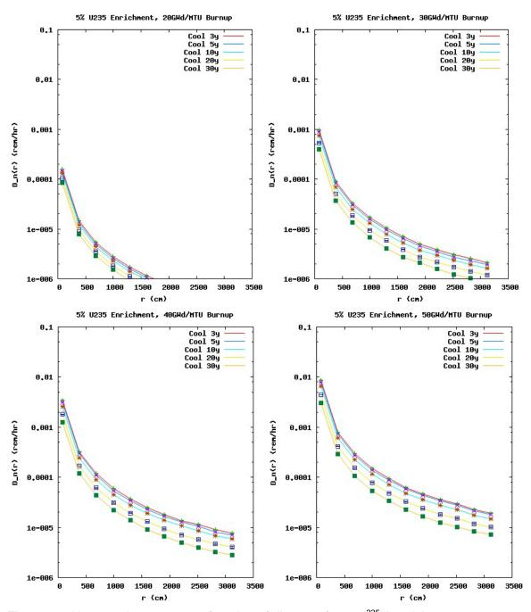
Figure 4. Neutron dose rate as a function of distance for 5% <sup>235</sup>U enrichment; 20, 30, 40, and 50 GWd/MTU burnup; and 3, 5, 10, 20, and 30 year cooling following irradiation.
