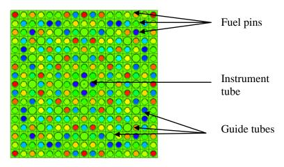
Figure 1. MCNP6 midplane fuel assembly geometry plot.
