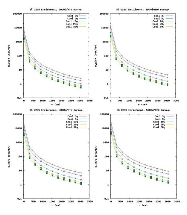
Figure 10. Photon dose rate as a function of distance for 3% <sup>235</sup>U enrichment; 20, 30, 40, and 50 GWd/MTU burnup; and 3, 5, 10, 20, and 30 year cooling following irradiation.
