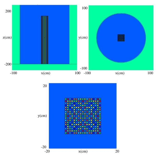
Figure 2. MCNP6 geometry plots of the 1.5-m-diameter chemical processing model showing fuel assembly, nitric acid (blue), and air (green).
