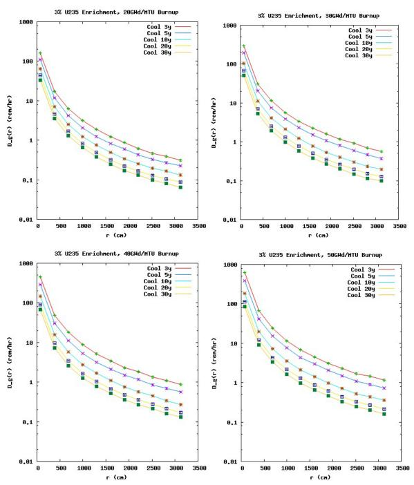
Figure 5. Photon dose rate as a function of distance for 3% <sup>235</sup>U enrichment; 20, 30, 40, and 50 GWd/MTU burnup; and 3, 5, 10, 20, and 30 year cooling following irradiation.
