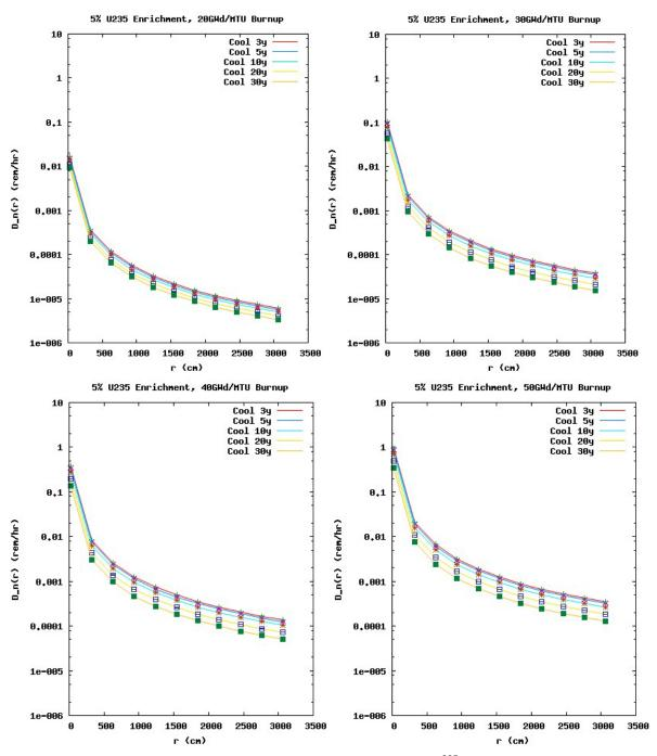
Figure 9. Neutron dose rate as a function of distance for 5% <sup>235</sup>U enrichment; 20, 30, 40, and 50 GWd/MTU burnup; and 3, 5, 10, 20, and 30 year cooling following irradiation.
