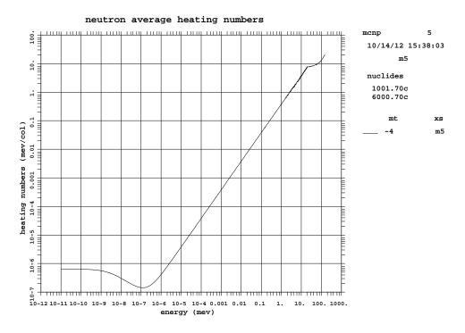
Figure 8: Exercise 6: Neutron heating of polyethylene.
