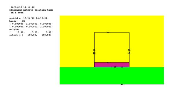
Figure 2: Exercise 1: Axial view of the can of plutonium nitrate solution.
