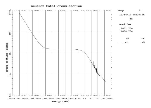
Figure 7: Exercise 6: Total neutron cross section of polyethylene.
