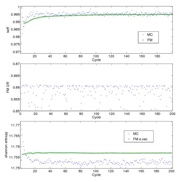
**Fig. 28.** Convergence behavior for the ATR problem, 100x100x1 spatial mesh. Fission matrix tallied for cycles 2-200, batch size of 1 M.
