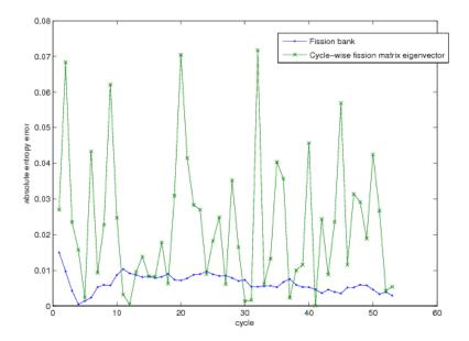
**Fig. 34** Absolute Shannon entropy errors for single-cycle fission bank and eigenvector of fission matrix tallied from single-cycle fission bank. 2D PWR problem, 30x30x1 spatial mesh, 500 k batch size.
