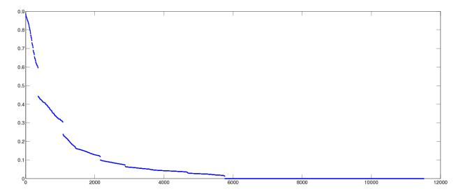
**Fig. 24.** Real part of the entire eigenvalue spectrum for the fuel storage vault problem, with 96x12x10 spatial mesh.
