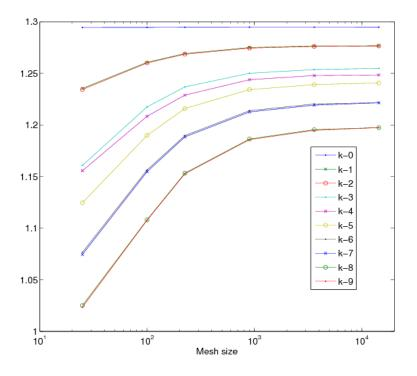
Fig. 5. Eigenvalue convergence behavior for increasingly fine meshing, 2D PWR problem.
