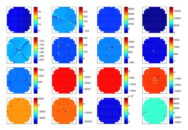
Fig. A.1. Percentage difference in sparse and full 0-15 eigenvectors for the 30x30x1 spatial mesh, 2D PWR problem:  $(s_{i,sparse}-s_{i,full})/s_{i,full}$ .
