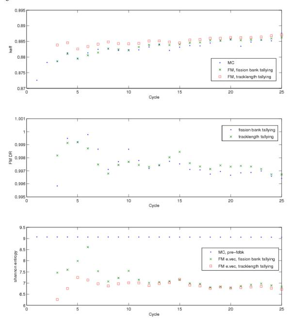
**Fig. 36.**  $k_{eff}$ , dominance ratio, and Shannon entropy convergence behavior for Monte Carlo, fission matrix with fission bank tallying, and fission matrix with track length tallying for fuel storage vault problem, 96x12x1 spatial mesh.
