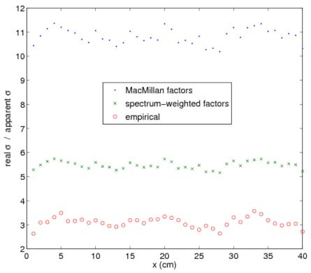
**Fig. 32.** MacMillan and spectrum weighted correction factors, along with empirical results for a 1D, 1-group problem.
