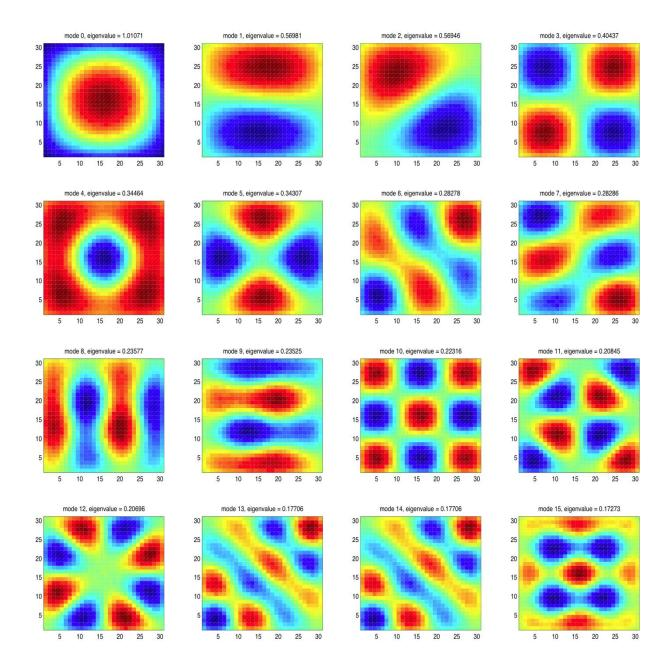
**Fig. A.4.** Higher eigenmodes for whole-core (30x30x1 spatial mesh) model of 2D homogenous reactor. Fission matrix tallied for 51 cycles, with batch size of 500 k.
