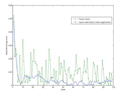
**Fig. 35** Absolute  $H_{src}$  errors for single-cycle fission bank and eigenvector of fission matrix tallied from single-cycle fission bank. 2D PWR problem, 10x10x1 spatial mesh, 500 k batch size.
