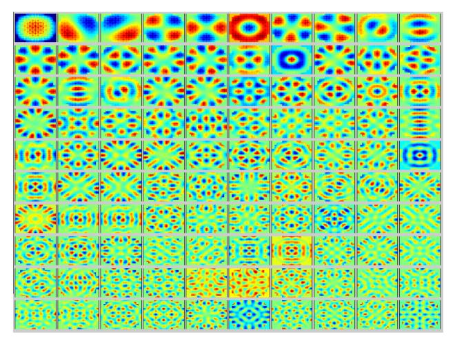
**Fig. A.3.** First 100 eigenmodes for 2D PWR problem on a 120x120x1 spatial mesh. Fission matrix tallied for 96 cycles with a batch size of 5 M.
