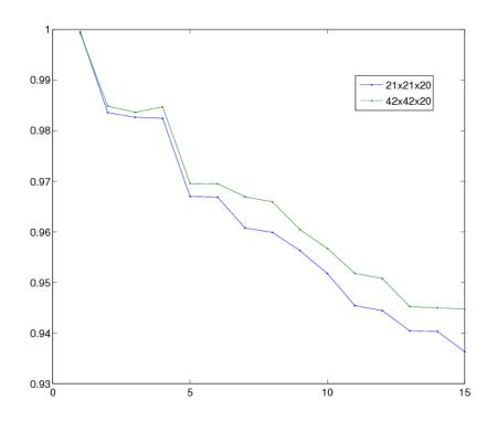
**Fig. 16.** First 15 eigenvalues (no imaginary components) of the Kord Smith Challenge, for two spatial mesh sizes: 21x21x20 and 42x42x20.
