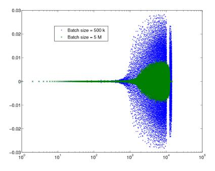
**Fig. 10.** Imaginary component of eigenvalue spectra for two batch sizes for the 120x120x1 spatial mesh, 2D PWR problem. Fission matrix tallied for cycles 4-100.
