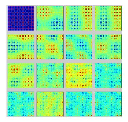
**Fig. D.6.** Real part of first 16 eigenmodes for infinite lattice of 2.1% enriched 17z17 assembly from 2D PWR problem. Fission matrix tallied for cycles 4-75, batch size of 500 k. 68x68x1 spatial mesh.
