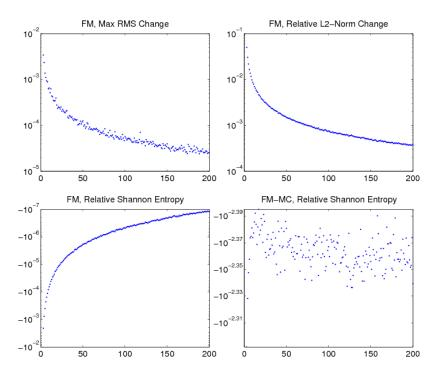
**Fig. 41** Various eigenvector convergence criteria, ATR Problem, 100 by 100, 1M batch size, fission matrix tallying begins cycle 2, solved every cycle
