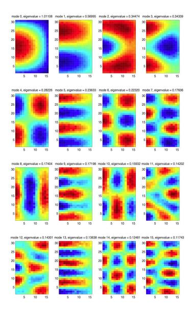
**Fig. A.5.** Higher eigenmodes for half-core (15x30x1 spatial mesh) model of 2D homogenous reactor. Fission matrix tallied for 51 cycles, with batch size of 500 k.
