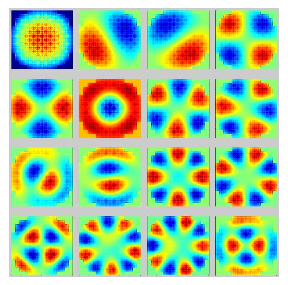
**Fig. 11** First 16 eigenmodes for 120x120x1 mesh, 2D PWR problem. Fission matrix tallied for cycles 4-100, with a batch size of 5 M.
