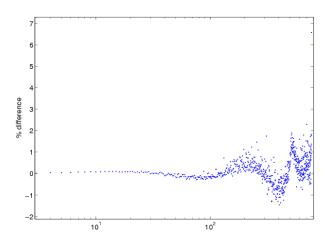
**Fig. 7.** Percentage difference in sparse and full eigenvalue spectra for the 30x30x1 spatial mesh, 2D PWR problem:  $(k_{i,sparse}-k_{i,full})/k_{i,full}$ .
