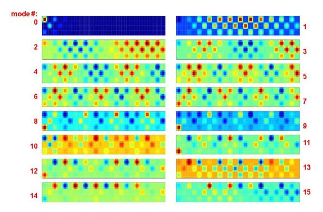
**Fig. 22.** First 16 eigenmodes of the fuel storage vault problem, with a 96x12x10 spatial mesh. Fission matrix tallied cycles 4-200, batch size of 1 M.
