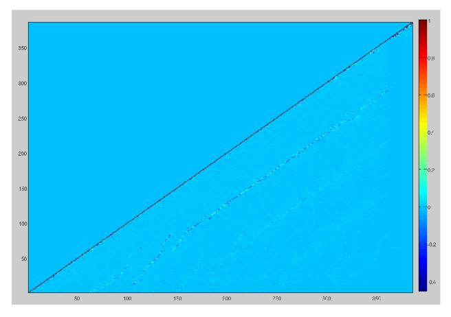
**Fig. C.1.** Magnitude of inner products (#n and #m) of first 385 forward eigenfunctions for fuel storage vault problem, 96x12x10 spatial mesh. Fission matrix tallied for cycles 3-200, 1 M batch size.
