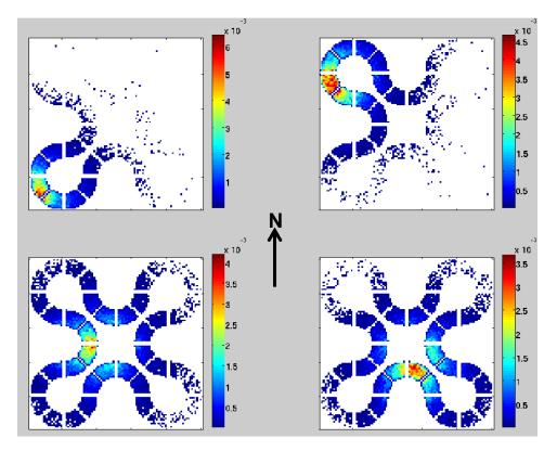
**Fig. 26.** Four full fission matrix columns for the ATR, 100x100x1 spatial mesh. Fission matrix tallied for cycles 2-200, batch size of 1 M.
