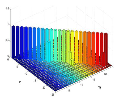
**Fig. 12.** Magnitude of inner products (#n and #m) of first 25 forward eigenfunctions for 2D PWR problem, 120x120x1 spatial mesh. Fission matrix tallied for cycles 4-100, 5 M batch size.
