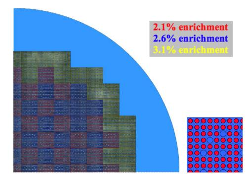
Fig. 2. Quadrant of whole-core, quarter-symmetric, PWR model, with section of 17x17 pin lattice shown.
