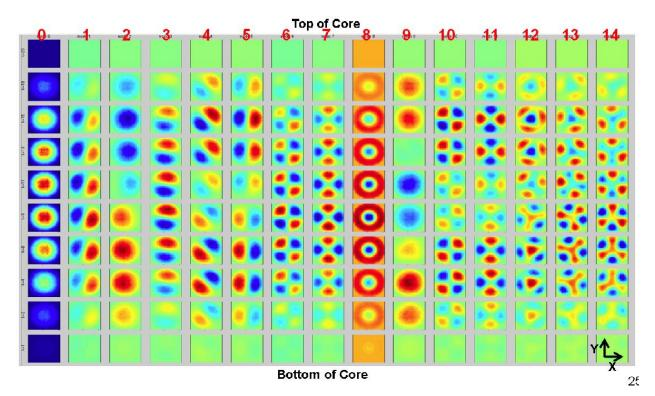
**Fig. 18.** First 15 eigenmodes for Kord Smith Challenge, 42x42x20 spatial mesh. Ten XY planes are shown. Fission matrix tallied for cycles 4-200, batch size of 1 M.
