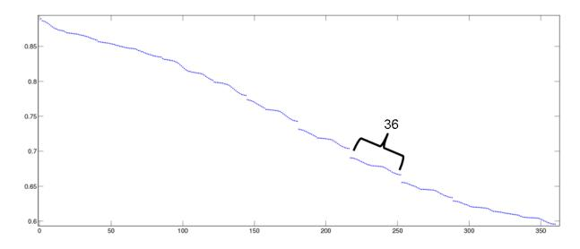
**Fig. 25.** Real part of the first 360 eigenvalues for the fuel storage vault problem, with 96x12x10 spatial mesh.
