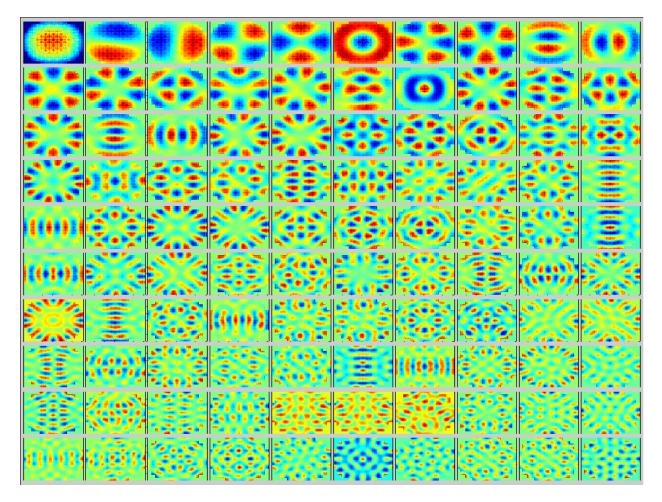
**Fig. A.2.** First 100 eigenmodes for 2D PWR problem on a 120x120x1 spatial mesh. Fission matrix tallied for 96 cycles with a batch size of 500 k.
