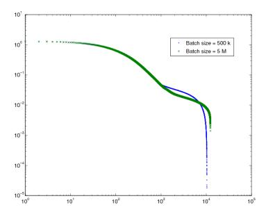
**Fig. 9.** Real component of eigenvalue spectra for two batch sizes for the 120x120x1 spatial mesh, 2D PWR problem. Fission matrix tallied for cycles 4-100.
