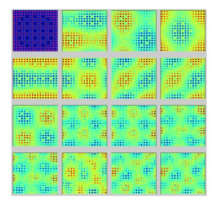
**Fig. D.5.** Real part of first 16 eigenmodes for infinite lattice of 2.1% enriched 17z17 assembly from 2D PWR problem. Fission matrix tallied for cycles 4-300, batch size of 500 k. 68x68x1 spatial mesh.
