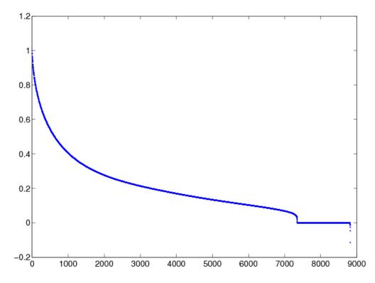
**Fig. 17.** Entire real part of the eigenvalue spectrum of the Kord Smith Challenge for the 21x21x20 spatial mesh.
