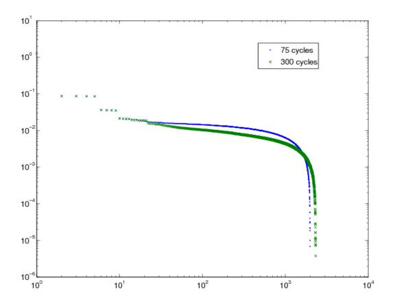
**Fig. D.3.** Real part of eigenvalue spectrum for infinite lattice of 2.1% enriched 17z17 assembly from 2D PWR problem. Fission matrix tallied for cycles 4-75 and 4-300, batch size of 500 k. 68x68x1 spatial mesh.
