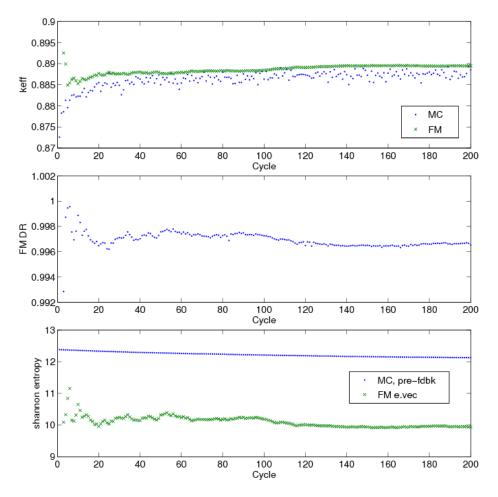
**Fig. 21.** Convergence behavior for the fuel storage vault problem, with a 96x12x10 spatial mesh. Fission matrix tallied cycles 3-200, batch size of 1 M.
