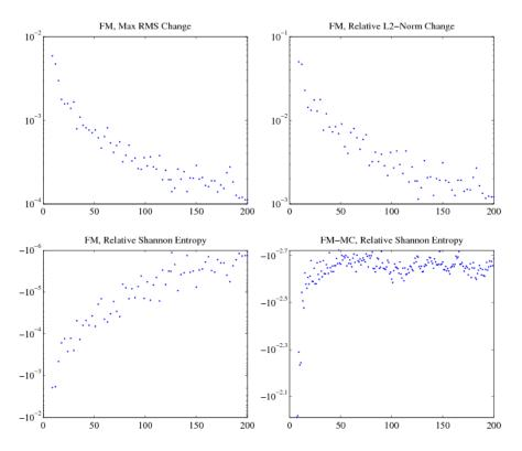
**Fig. 38** Various eigenvector convergence criteria, 2D PWR, 30 by 30, 500k batch size, fission matrix tallying begins cycle 4, solved every 3 cycles
