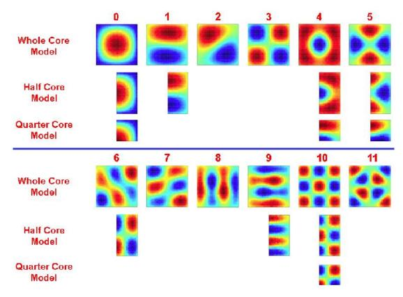
**Fig. 13.** Higher eigenmodes for whole-core (30x30x1 spatial mesh), half-core (15x30x1 spatial mesh), and quarter-core (15x15x1 spatial mesh) models of 2D homogenous reactor. Fission matrices tallied for cycles 4-55, with batch size of 500 k.
