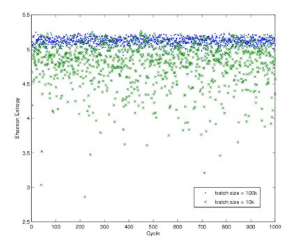
**Fig. 33.** Single-cycle fission matrix eigenvector Shannon entropy for 100k and 10k batch sizes. 1D, 1-group problem, 40 cm, 40x1x1 spatial mesh, 1000 cycles ran.
