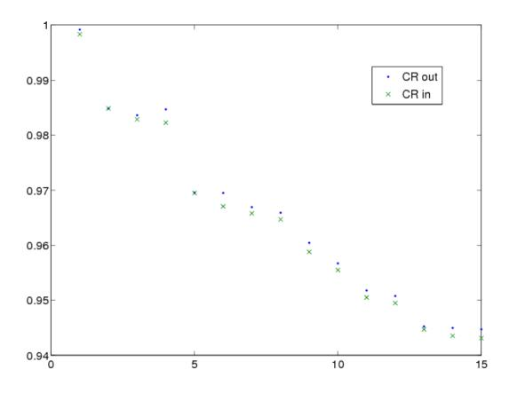
**Fig. B.2.** First 15 eigenvalues for Kord Smith Challenge with Silver-Indium-Cadmium control rods [17] fully inserted into one assembly., 42x42x20 spatial mesh. Also shown are first 15 eigenvalues with control rod insertion. Fission matrix tallied for cycles 4-200, batch size of 1 M.
