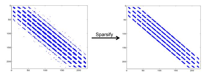
**Fig. 1.** Fission matrix structure for a 2D whole-core PWR model, for a 15x15x1 spatial mesh. Matrix dimension are 225 x 225. Nonzero elements are in blue.
