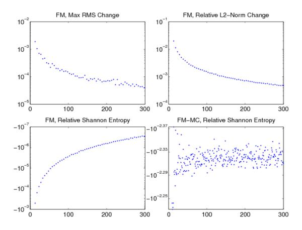
**Fig. D.2.** Convergence metrics for infinite lattice of 2.1% enriched 17z17 assembly from 2D PWR problem. Fission matrix tallied for cycles 4-300, batch size of 500 k. 68x68x1 spatial mesh.
