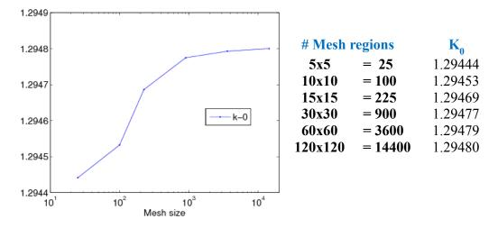
Fig. 6. Fundamental eigenvalue convergence behavior for increasingly fine meshing, 2D PWR problem.
