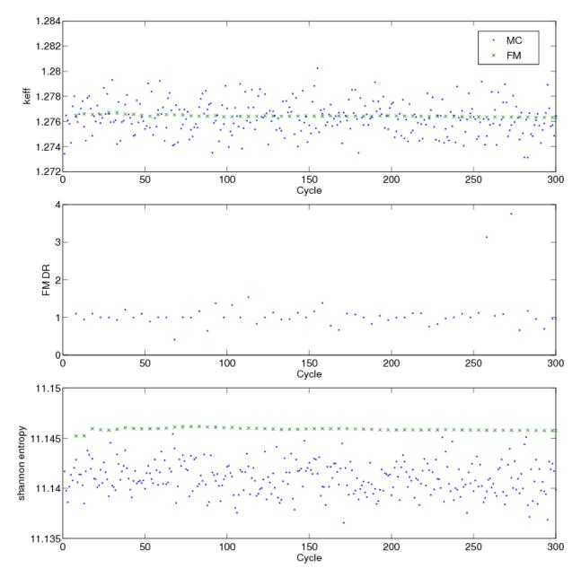
**Fig. D.1.** Convergence behavior for infinite lattice of 2.1% enriched 17z17 assembly from 2D PWR problem. Fission matrix tallied for cycles 4-300, batch size of 500 k. 68x68x1 spatial mesh.
