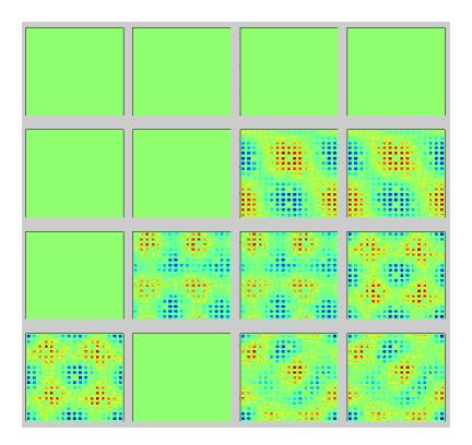
**Fig. D.7.** Imaginary part of first 16 eigenmodes for infinite lattice of 2.1% enriched 17z17 assembly from 2D PWR problem. Fission matrix tallied for cycles 4-300, batch size of 500 k. 68x68x1 spatial mesh.
