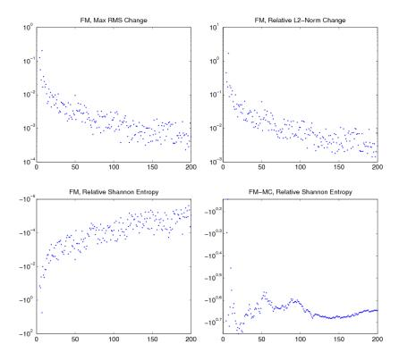
**Fig. 40** Various eigenvector convergence criteria, Fuel Storage Vault Problem, 96 by 12 by 10, 1M batch size, fission matrix tallying begins cycle 3, solved every cycle
