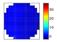
Fig. 8. Percentage difference in sparse and full fundamental eigenvectors for the 30x30x1 spatial mesh, 2D PWR problem:  $(s_{i,sparse}-s_{i,full})/s_{i,full}$ .
