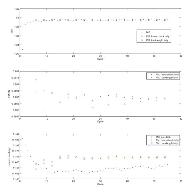
**Fig. 37.**  $k_{eff}$ , dominance ratio, and Shannon entropy convergence behavior for Monte Carlo, fission matrix with fission bank tallying, and fission matrix with tracklength tallying for 2D PWR problem, 60x60x1 spatial mesh.
