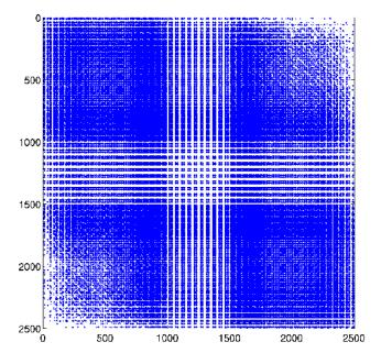
**Fig. 27.** Fission matrix structure for 50x50x1 spatial mesh, ATR problem. Fission matrix tallied for cycles 2-100, batch size of 500 k.
