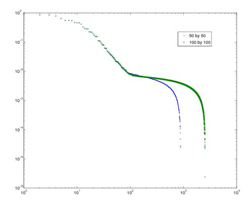
Fig. 31. Eigenvalue spectrums of the ATR problem, with a 100x100x1 spatial mesh.
