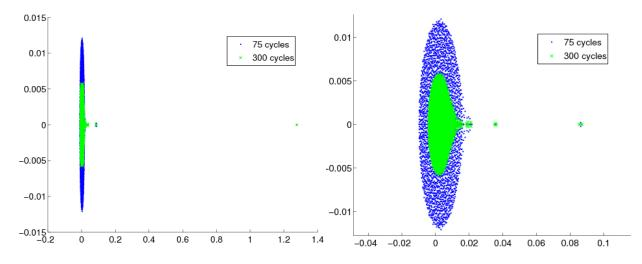
**Fig. D.4.** Eigenvalue spectrum on complex plane (two scales) for infinite lattice of 2.1% enriched 17z17 assembly from 2D PWR problem. Fission matrix tallied for cycles 4-75 and 4-300, batch size of 500 k. 68x68x1 spatial mesh.
