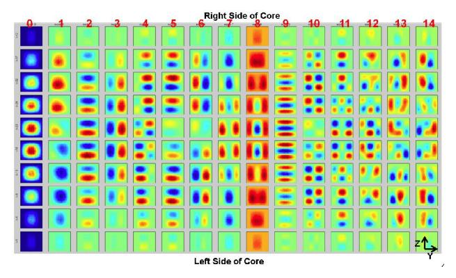
**Fig. 19.** First 15 eigenmodes for Kord Smith Challenge, 42x42x20 spatial mesh. Ten YZ planes are shown. Fission matrix tallied for cycles 4-200, batch size of 1 M.
