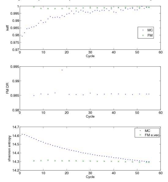
**Fig. 14.** Fundamental eigenvalue, dominance ratio estimate from fission matrix power iteration, and Shannon entropy convergence behavior for unaffected Monte Carlo fission bank and fission matrix eigenvector. Kord Smith Challenge, 42x42x20 spatial mesh. Fission matrix tallied for cycles 4-55, batch size of 1 M.
