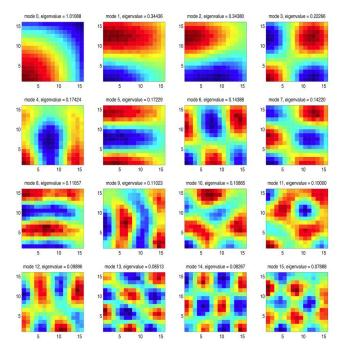
**Fig. A.6.** Higher eigenmodes for quarter-core (15x15x1 spatial mesh) model of 2D homogenous reactor. Fission matrix tallied for 51 cycles, with batch size of 500 k.
