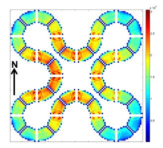
**Fig. 29.** Fundamental eigenvector of the fission matrix with 100x100x1 spatial mesh, ATR problem. Fission matrix tallied for cycles 2-200, batch size of 1M.
