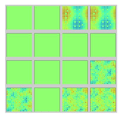
**Fig. D.8.** Imaginary part of first 16 eigenmodes for infinite lattice of 2.1% enriched 17z17 assembly from 2D PWR problem. Fission matrix tallied for cycles 4-75, batch size of 500 k. 68x68x1 spatial mesh.
