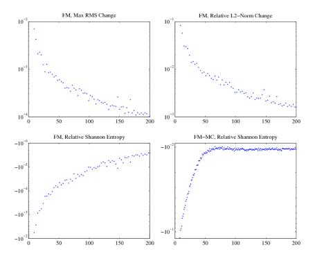
**Fig. 39** Various eigenvector convergence criteria, 3D Kord Smith Challenge Problem, 21 by 21 by 20, 1M batch size, fission matrix tallying begins cycle 4, solved every 3 cycles
