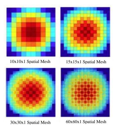
**Fig. 3.** 2D PWR fundamental eigenmodes for 4 spatial meshes. Fission matrix tallied for cycles 4-55, with a batch size of 500 k.
