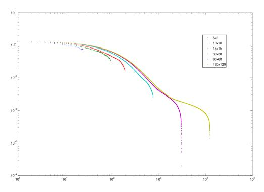
Fig. 4. Real component of eigenvalue spectrum for 2D PWR problem. Six different spatial resolutions are shown.
