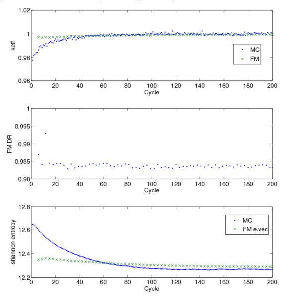
**Fig. 15.** Fundamental eigenvalue, dominance ratio estimate from fission matrix power iteration, and Shannon entropy convergence behavior for unaffected Monte Carlo fission bank and fission matrix eigenvector. Kord Smith Challenge, 21x21x20 spatial mesh. Fission matrix tallied for cycles 4-200, batch size of 1 M.
