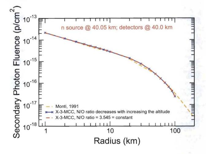
Figure 4: Secondary photon fluence at 40 km from a source at 40.05 km vs. radius (slant range) calculated with the standard, unmodified MCNP6 for the geometry shown on Fig. 1 using a Nitrogen-to-Oxygen ratio for the air decreasing with the increase of the altitude according to the U.S. Standard Atmosphere Tables, 1976 [16] (solid blue line) and using a constant, sea-level, N/O ratio (red dashed line) compared with results by Monti with a modification of MCNP3B [11] (orange dashed line).
