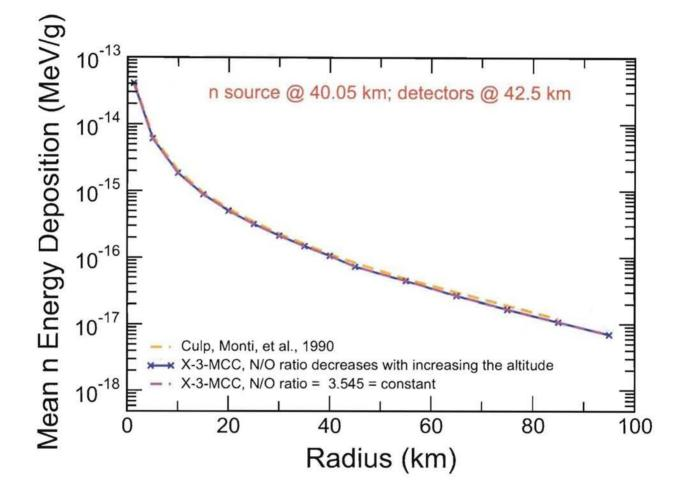
Figure 3: Mean neutron energy deposition at 42.5 km from a source at 40.05 km vs. radius (slant range) calculated with the standard, unmodified MCNP6 for the geometry shown on Fig. 3 using a Nitrogen-to-Oxygen ratio for the air decreasing with the increase of the altitude according to the U.S. Standard Atmosphere Tables, 1976 [16] (solid blue line) and using a constant, sea-level, N/O ratio (red dashed line) compared with unmodified MCNP3B results by Culp et al., [17] (orange dashed line.
