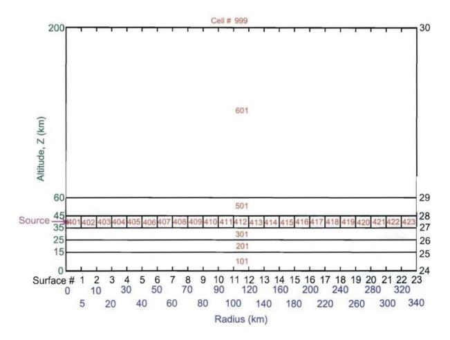
Figure 8: Spatial cell geometry for the co-altitude test problems with the modified here MCNP6.
