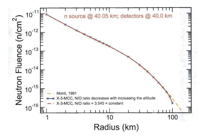
Figure 2: Neutron fluence at 40 km from a source at 40.05 km vs. radius (slant range) calculated with the standard, unmodified MCNP6 for the geometry shown on Fig. 1 using a Nitrogento-Oxygen ratio for the air decreasing with the increase of the altitude according to the U.S. Standard Atmosphere Tables, 1976 [16] (solid blue line) and using a constant, sea-level, N/O ratio (red dashed line) compared with results by Monti with a modification of MCNP3B [11] (orange dashed line).
