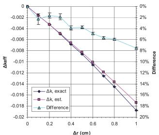
Fig. 4. The change in  $k_{eff}$  as a function of the "collapsing" displacement of the left side of the <sup>235</sup>U sphere.
