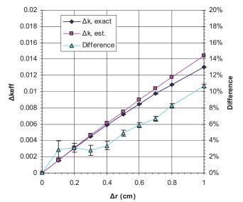
Fig. 3. The change in  $k_{eff}$  as a function of the "bulging" displacement of the right side of the <sup>235</sup>U sphere.
