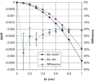
Fig. 2. The change in  $k_{eff}$  as a function of the translation of the <sup>235</sup>U sphere. 1 $\sigma$  error bars are shown in all figures.
