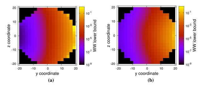
Figure 5. Linear tally combination lower weight-window bounds in concrete sphere for (a) plane tallies through sphere, and (b) a mesh tally .
