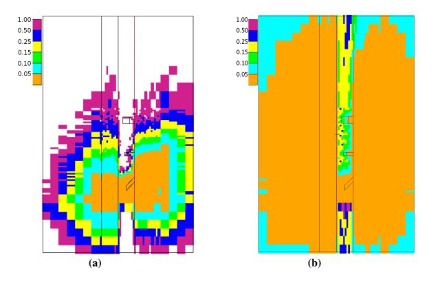
Figure 9. (a) Voxel relative error after default mesh tally production run of  $1 \times 10^8$  histories, and (b) voxel relative error after mesh tally weight-window generation using linear tally combination and production run of  $5 \times 10^7$  histories.
