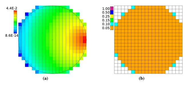
Figure 6. Mesh tally (a) values and (b) relative error after generation of weight windows using the mesh tally on the linear tally combination.
