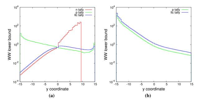
Figure 7. (a) neutron and (b) photon weight windows as a function of the tally being optimized .
