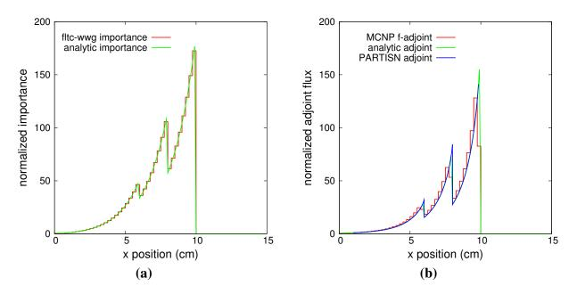
Figure 3. (a) Comparison of the spatial analytic importance function to the importance function generated using MCNP's weight-window generator and the linear tally combination, and (b) a similar comparison of the adjoint fluxes. All results are normalized to unity in the cell containing the physical source.
