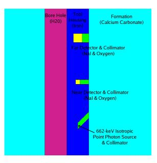
Figure 8. gamma-gamma density oil-well logging tool model geometry.
