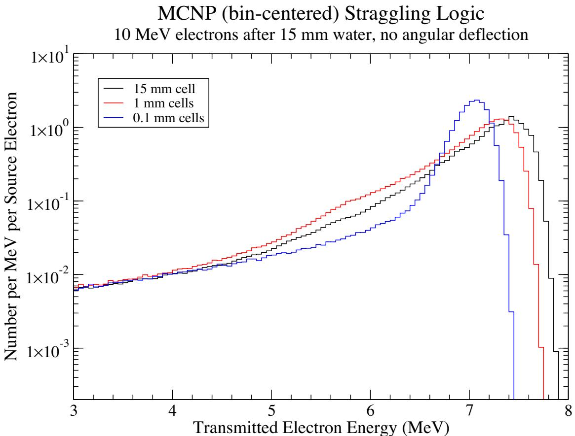
**Figure 1. Results of the bin-centered straggling logic for three equivalent geometries showing unphysical step-size artifacts.**
