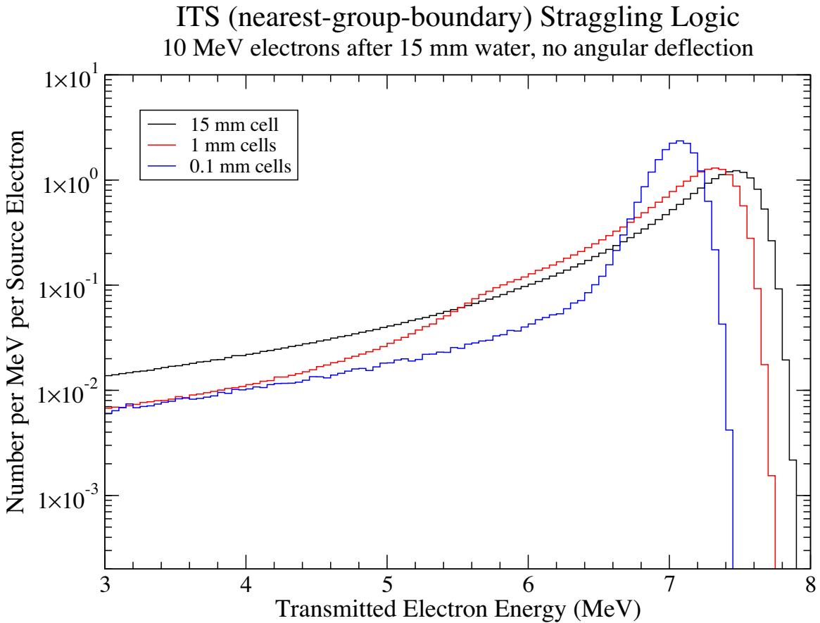
**Figure 2. Results of the nearest-group-boundary straggling logic for three equivalent geometries again showing unphysical step-size artifacts.**
