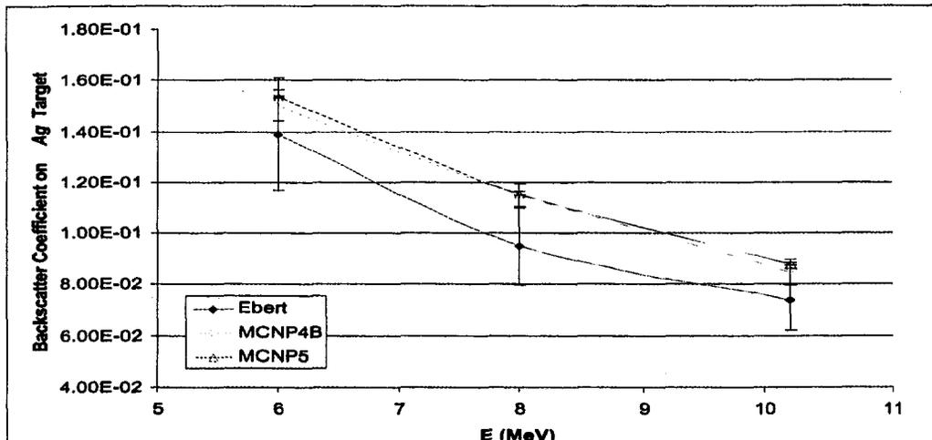
Figure 5. Electron backscatter coefficient through elemental *Ag* target.
