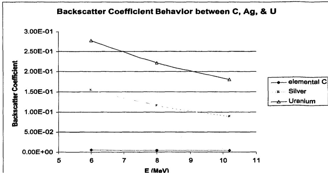
**Figure 8. Backscatter Coefficient on Elemental Carbon, Silver, and Uranium**
