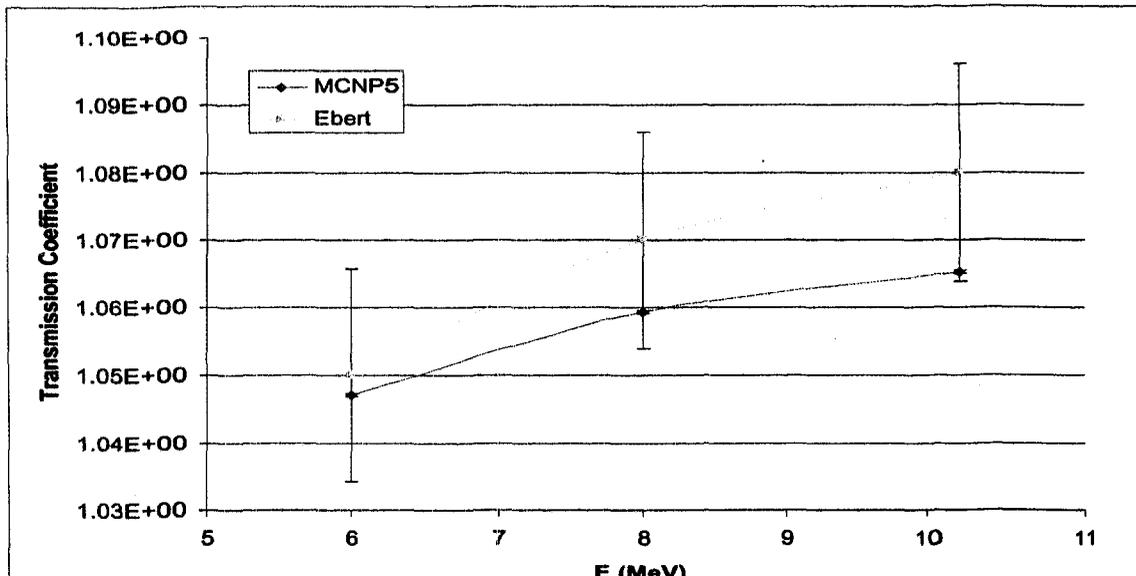
Figure 3. Electron transmission coefficient through elemental C target.
