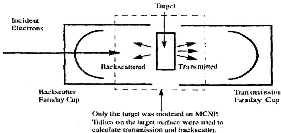
Figure 1. Geometry of Ebert transmission and backscatter experiments.
