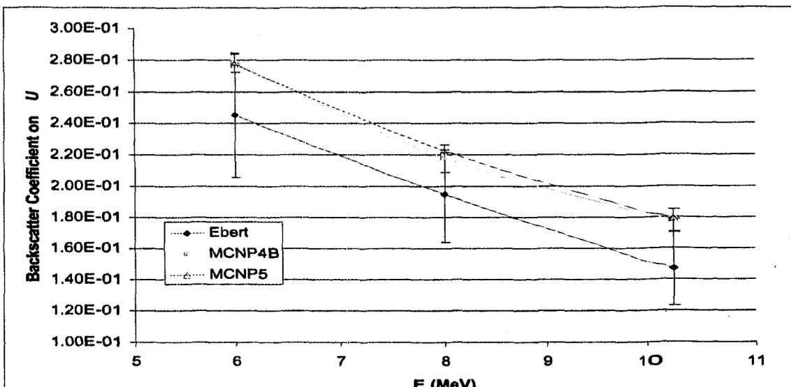
Figure 6. Electron backscatter coefficient through elemental U target.
