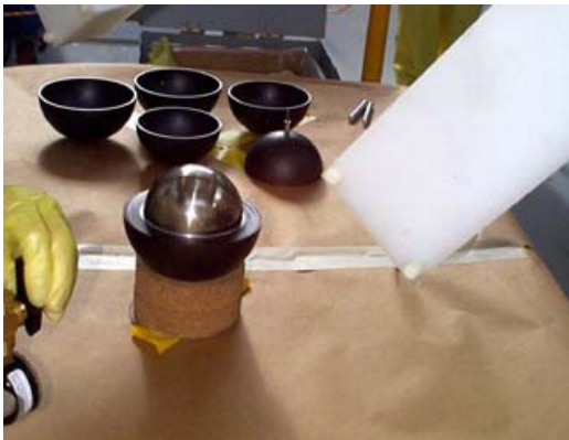
Fig. 2 Neptunium sphere surrounded with HEU shells.
