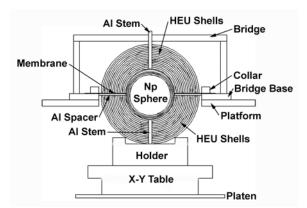
Fig. 1. Schematic of the Experiment.
