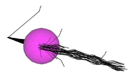
Figure 1. Perspective view, slightly off the beam axis, of the radiographed object (22.5 cm radius) and 100 proton tracks (9940 cm length along the axis). The wobbles in the proton tracks are caused by the COSY maps simulating the focusing effect of the quadrupole magnets. The diffuser and collimators are not shown.
