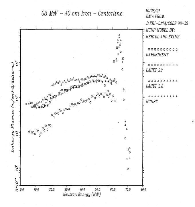
Fig. 1. Comparison of LAHET 2.7, LAHET 2.8 and MCNPX with experimental results in the JAERI experiment. The transmitted neutron fluence is measured and calculated immediately adjacent to the down-stream side of the iron transmission target directly on the beam centerline.
