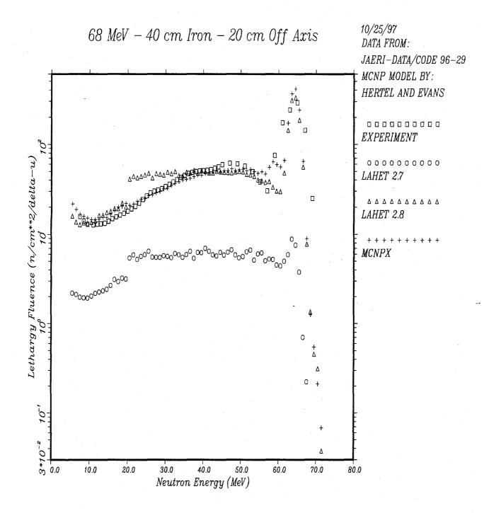
Fig. 2. Comparison of LAHET 2.7, LAHET 2.8 and MCNPX with experimental results in the JAERI experiment. The transmitted neutron fluence is measured and calculated immediately adjacent to the down-stream side of the iron transmission target at a position 20 cm away from the beam centerline.
