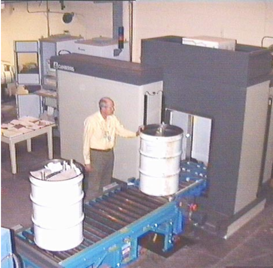
Fig. 3.9. Top view of the High Efficiency Neutron Counter developed by Los Alamos National Laboratory and Canberra Industries.
