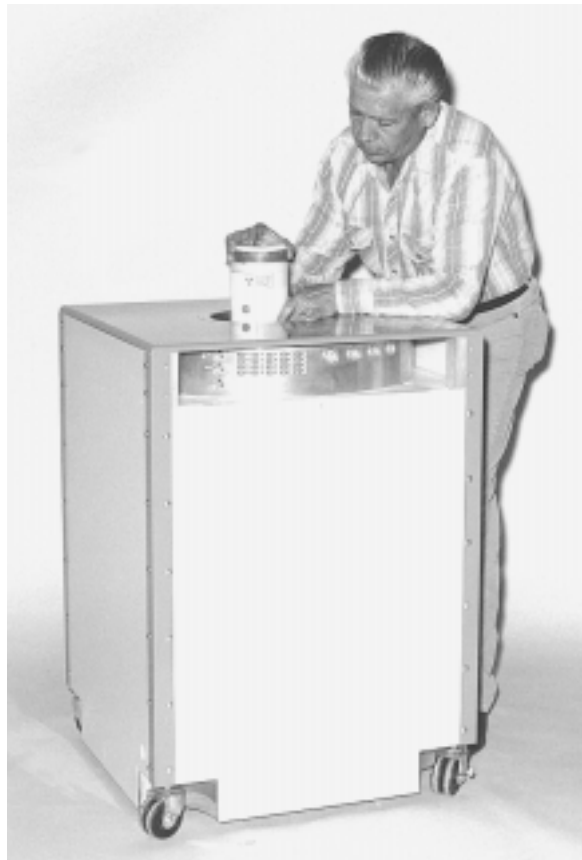
Fig. 1.1. Photo of the Plutonium Scrap Multiplicity Counter, used for accurate assays of cans of plutonium metal, oxide, mixed oxide, or scrap.
