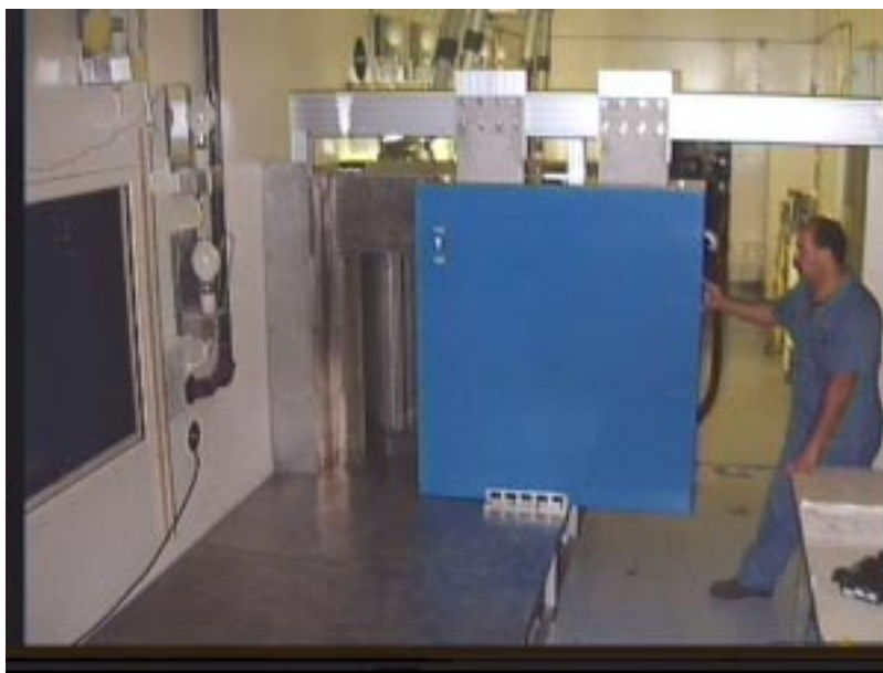
Fig. 3.8. The Shield Cell Drum Neutron Counter, with multiplicity, shuffler, and add-a-source capability.
