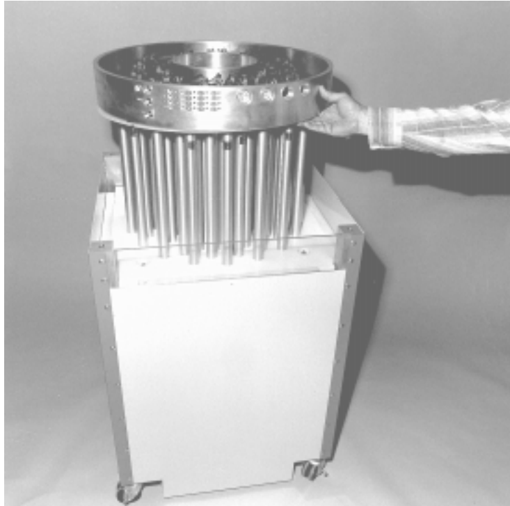
Fig. 3.3. Photograph of the ^3\text{He} tubes and high-voltage junction box partly withdrawn from the Plutonium Scrap Multiplicity Counter.
