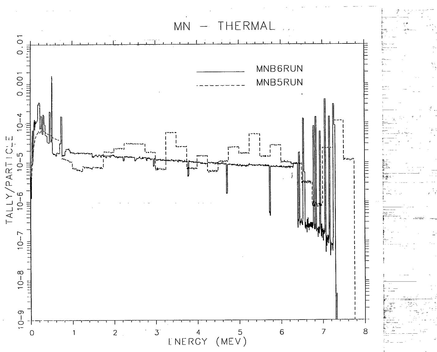
Figure 10: Photon Production for Mn at Incident Thermal Neutron Energies.
