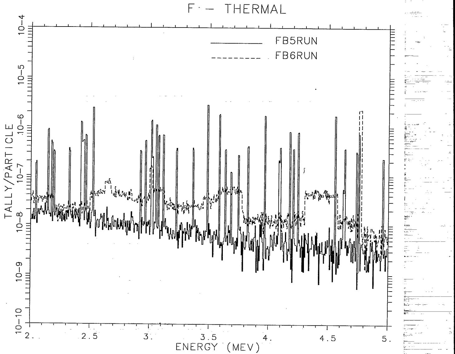
Figure 4: Photon Production for  $^{19}\text{F}$  at Incident Thermal Neutron Energies.
