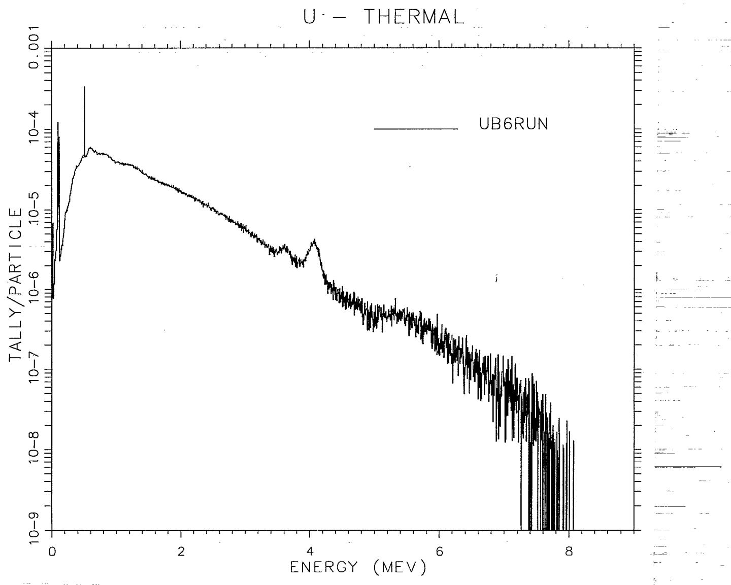
Figure 3: Photon Production for U at Incident Thermal Neutron Energies.
