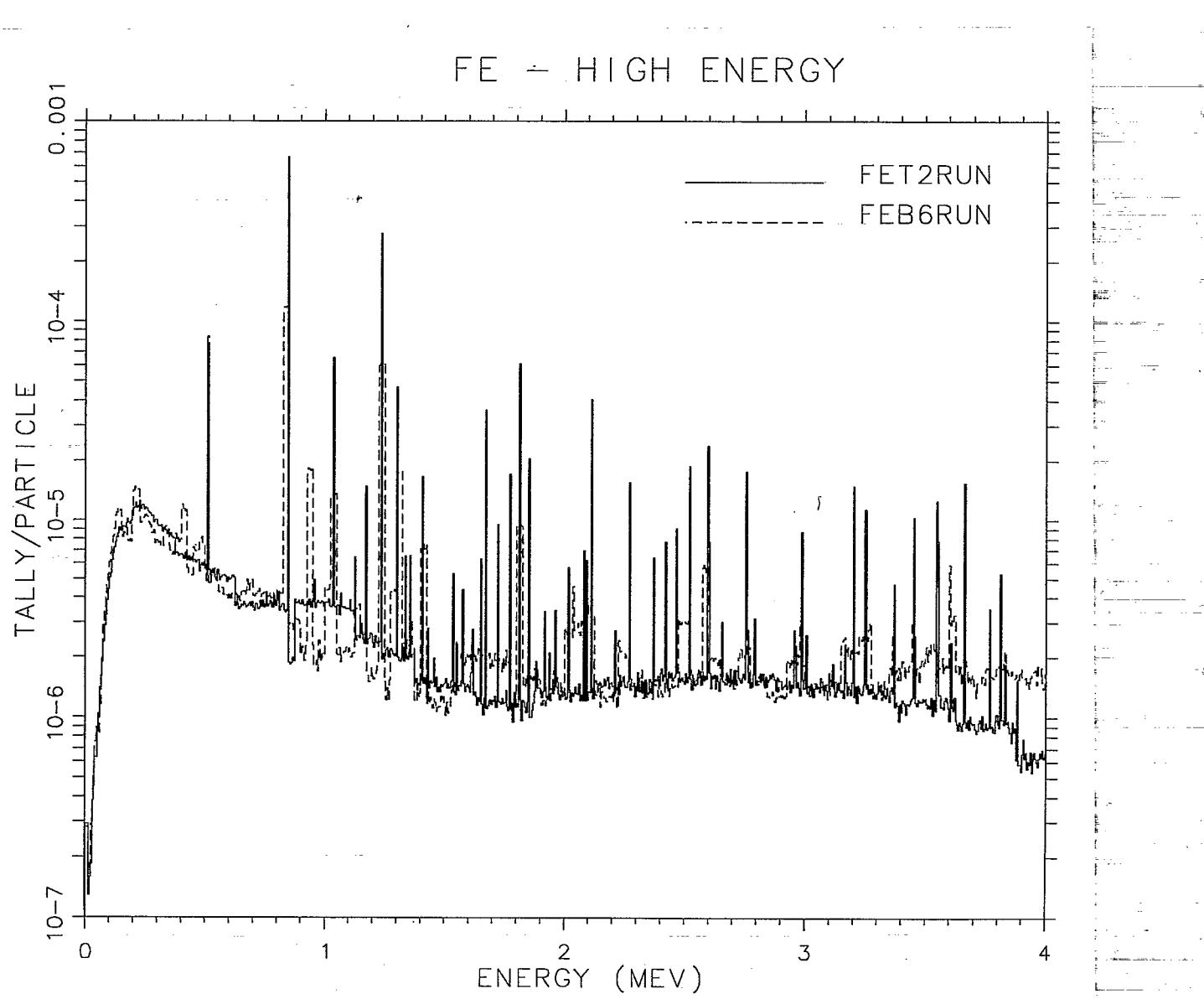
Figure 6: Photon Production for Fe at 14-MeV Incident Neutron Energies.
