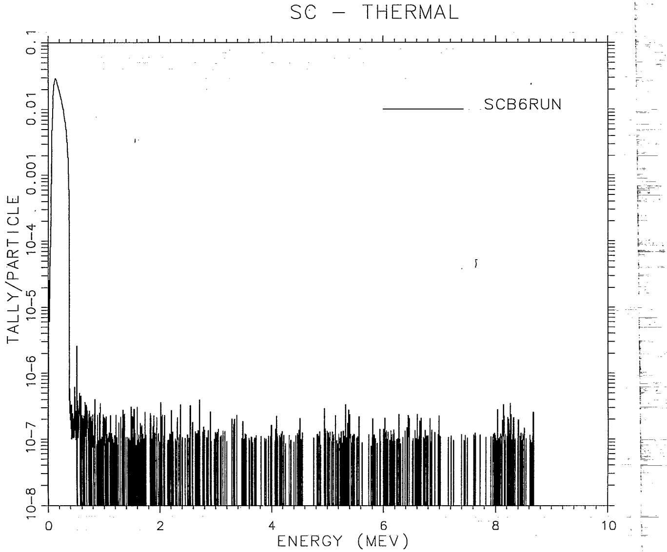
Figure 8: Photon Production for Sc at Incident Thermal Neutron Energies.
