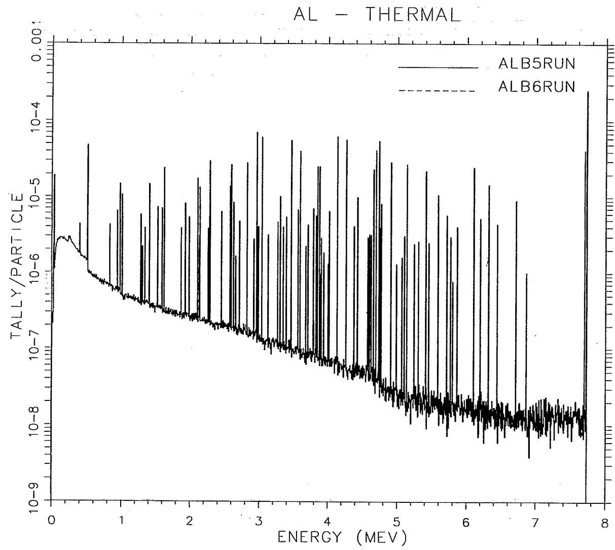
Figure 1: Photon Production for Al at Incident Thermal Neutron Energies.
