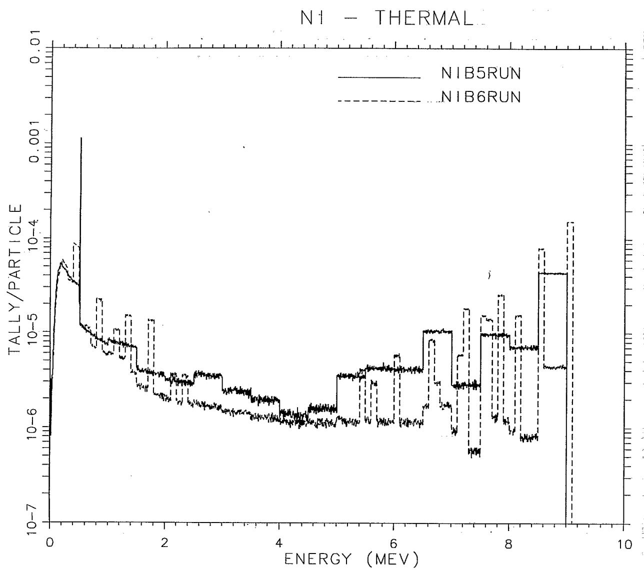
Figure 11: Photon Production for Ni at Incident Thermal Neutron Energies.
