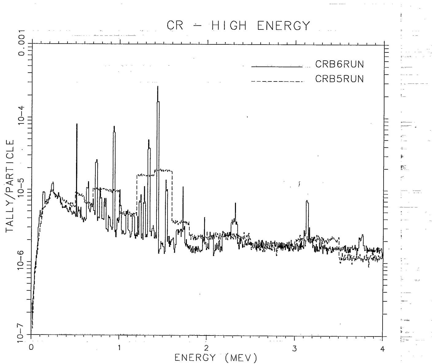
Figure 7: Photon Production for Cr at 14-MeV Incident Neutron Energies.
